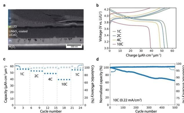
Fig. 13 (a) Cross-section SEM image of the battery stack. (b) Charge-discharge curves at different C rates (1C =  $22 \mu\text{A cm}^{-2}$ ). (c) Discharge capacity and coulombic efficiency of the battery at different C rates. (d) Long-term cycling of the battery over 500 cycles at 10C (0.22  $\text{mA cm}^{-2}$ ).<sup>160</sup> Copyright 2021 Springer Nature Limited.
