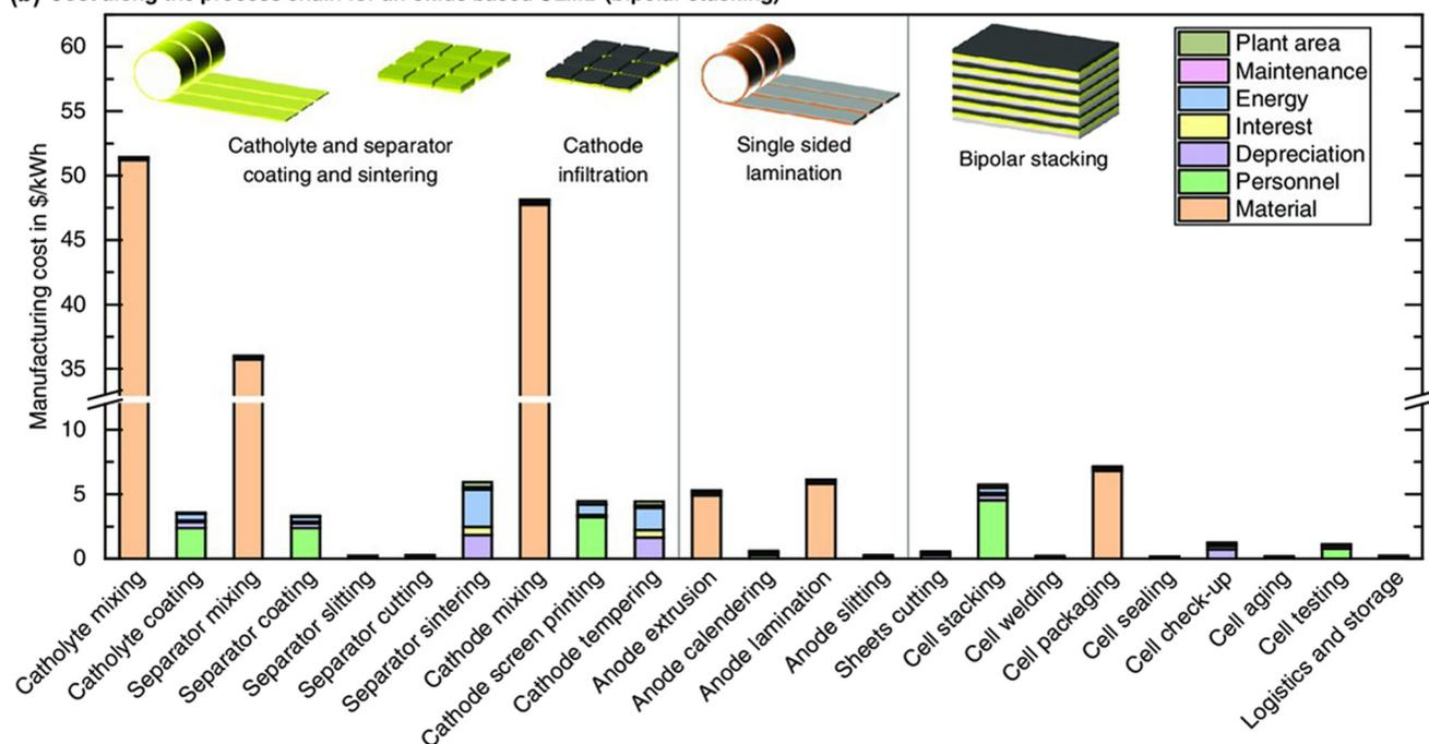
Fig. 15 Manufacturing cost along the process chains for (a) sulfide- and (b) oxide-based solid-state lithium metal batteries (SLMB) for a production output of 6 GW h per year.<sup>190</sup> Copyright 2020, John Wiley and Sons.
