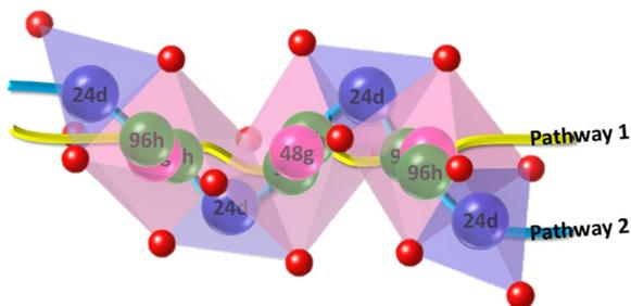
**Fig. 4** The lithium diffusion pathway in the cubic LLZO crystal. The diffusion follows two paths. Pathway 1: 96h–48g–96h–48g–96h involving only octahedral sites (yellow line). Pathway 2: 24d–96h–48g–96h–24d involving both octahedral and tetrahedral sites (blue line).
