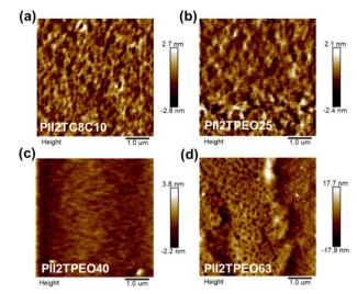
Fig. 5 AFM height images of the isoindigo-based polymer films of PII2TC8C10, (b) PII2TPEO25, (c) PII2TPEO40, PII2TPEO63, respectively.
