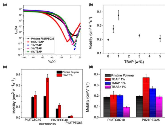
**Fig. 3** FET characteristics of the studied polymers under different conditions: (a) transfer curves of the studied polymer films; (b) PII2TPEO25 doped with different ratios of TBAP; (c) different ratios of alkoxy side-chain conjugated polymers doped with 1% of TBAP; (d) PII2TC8C10 and PII2TPEO25 doped with different ionic additives.
