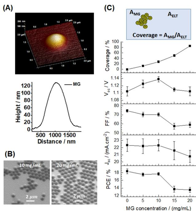
Fig. 2 (A) A 3D AFM perspective image and a line profile for a representative MG particle. (B) SEM images of MGs deposited on glass/ITO/SnO<sub>2</sub> using two concentrations. (C) Coverage and PSC performance parameter variation with MG concentration used.  $A_{MG}$  and  $A_{ETL}$  are the total areas of the MGs and ETL.
