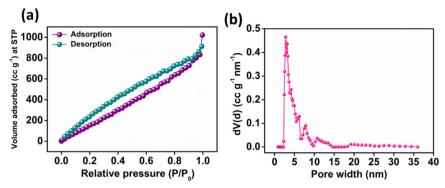
Fig. 3 (a) N<sub>2</sub> adsorption-desorption plot and (b) pore size distribution curve of N-CA.
