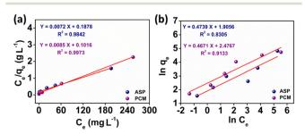
Fig. 6 Plot of the adsorption isotherms of ASP and PCM: (a) Langmuir and (b) Freundlich.
