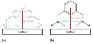
Fig. 3 Definitions of configurational descriptors used for investigating the binding modes of (a) DGEBA and (b) MXDA to surfaces.
