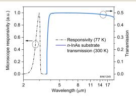
Fig. 1 Spectral responsivity of the IR microscope/camera at 77 K (left scale) and the estimated optical transmission of a 100 µm-thick n-InAs substrate (right scale).
