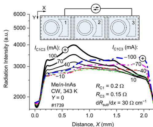
**Fig. 5** Thermal radiation intensity  $L(x, y)$  at the  $n$ -InAs surface vs. the distance along the symmetry axis  $X$  ( $Y = 0$ ) with two directions of current: from left to right (solid lines) and from right to left (dashed lines).
