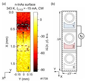
Fig. 4 (a) False IR image of the troika surface activated by current  $I_{C1C2} = -15$  mA (see vertical arrow indicating current direction) together with the areas above the anodes (dashed lines) and  $\Delta L(x, y)$ color scale on the right; (b) troika schematic (top n-InAs substrate view) with projections of mesas, separation grooves, contacts (all dashed lines) and the area for analysis  $\Delta X \Delta Y$  (dashed line).
