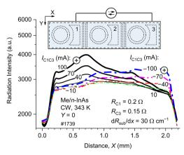
Fig. 5 Thermal radiation intensity L(x, y) at the n-InAs surface vs. the distance along the symmetry axis X (Y = 0) with two directions of current: from left to right (solid lines) and from right to left (dashed
