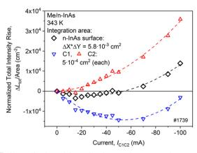
Fig. 7 Normalized total intensity rise vs. the current  $I_{C1C2}$  at three integration areas: above the contacts C1 and C2 (triangles) and above the (100) n-InAs surface (clubs)
