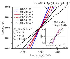
Fig. 3 I-V characteristics at 77 K (solid lines) and 300 K (dashed lines) for three connection types: C1-C2 (blue), C2-C3 (red) and C1-C3 (black). The insert shows I-V characteristics at the bias up to  $\pm 1 \text{ V}$ .
