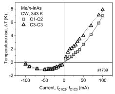
Fig. 6 Maximum temperature rise  $\Delta T$  in the contact regions C1 ( $X = \frac{1}{2}$ ) 0.35-0.5 mm) in the contact pair C1-C2 (squares) and C3 in the pair C1-C3 (X = 1.6-1.75 mm) vs. current.
