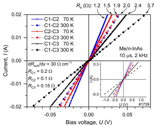
**Fig. 3**  $I$ - $V$  characteristics at 70 K (solid lines) and 300 K (dashed lines) for three connection types: C1-C2 (blue), C2-C3 (red) and C1-C3 (black). The insert shows  $I$ - $V$  characteristics at the bias up to  $\pm 1$  V.
