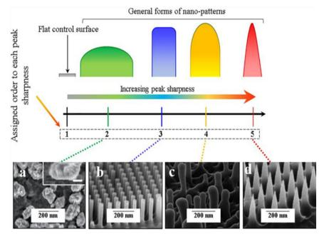
Fig. 9 Illustrations of different forms of the peak sharpness and their assigned orders in this study compared to the flat control surface and examples of the corresponding shapes in the literature (a) nano-nuggets (magnified SEM image is given in the inset, scale bar: 50nm), (b) nanopillars, (c) nanopillar (of dragonfly wing) and (d) nano-spikes. 78 Copyright 2021, Elsevier.
