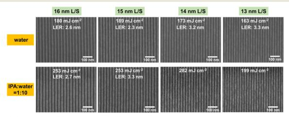
Fig. 7 The 16, 15, 14 and 13 nm L/S line patterns of the SnMSF<sub>4</sub> resists developed with water and the mixture of IPA and H<sub>2</sub>O ( $V_{IPA}$ :  $V_{H-O}$  = 1:10).
