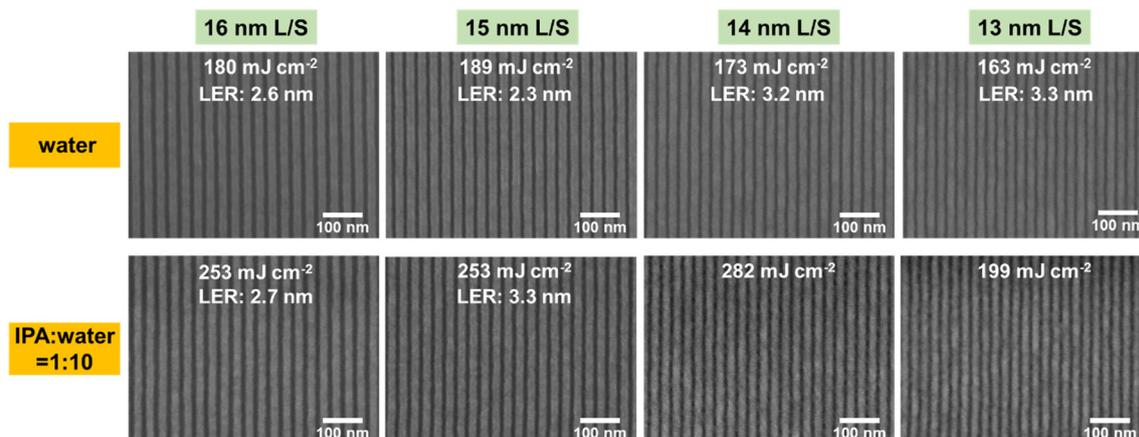
Fig. 7 The 16, 15, 14 and 13 nm L/S line patterns of the SnMSF<sub>4</sub> resists developed with water and the mixture of IPA and H<sub>2</sub>O ( $V_{\text{IPA}}:V_{\text{H}_2\text{O}} = 1:10$ ).
