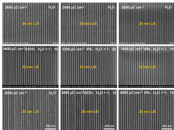
Fig. 6 The patterns of SnMSF<sub>4</sub> resists for EBL.
