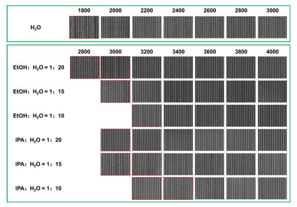
Fig. 5 The 22 nm L/S patterns of the SnMSF<sub>4</sub> resist developed in the different developers for EBL
