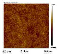
Fig. 3 AFM image of the SnMSF<sub>4</sub> resist film.
