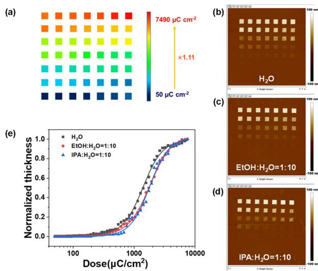
Fig. 4 The sensitivity and contrast analysis of SnMSF<sub>4</sub> for e-beam exposure. (a) The e-beam exposure layout for NRT testing. (b–d) AFM images of SnMSF<sub>4</sub> patterns developed with H<sub>2</sub>O, the EtOH/H<sub>2</sub>O mixture (*V*<sub>EtOH</sub>:*V*<sub>H<sub>2</sub>O</sub> = 1:10) and the IPA/H<sub>2</sub>O mixture (*V*<sub>IPA</sub>:*V*<sub>H<sub>2</sub>O</sub> = 1:10). (e) The NRT curves of the SnMSF<sub>4</sub> resist.
