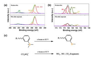
Fig. 8 (a) C 1s and (b) S 2p XPS core spectra of the SnMSF<sub>4</sub> resist films before and after e-beam exposure. (c) Proposed decomposition process of sulfonium and CF<sub>3</sub>SO<sub>3</sub> units.
