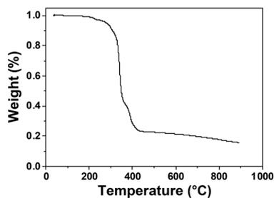
Fig. 2 TGA curve of SnMSF<sub>4</sub> at a heating rate of 10 °C min<sup>-1</sup> under an N<sub>2</sub> atmosphere.
