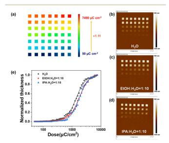
Fig. 4 The sensitivity and contrast analysis of SnMSF<sub>4</sub> for e-beam exposure. (a) The e-beam exposure layout for NRT testing. (b–d) AFM images of SnMSF<sub>4</sub> patterns developed with H<sub>2</sub>O, the EtOH/H<sub>2</sub>O mixture ( $V_{\rm EtOH}:V_{\rm H_2O}=1:10$ ) and the IPA/H<sub>2</sub>O mixture ( $V_{\rm IPA}:V_{\rm H_2O}=1:10$ ). (e) The NRT curves of the SnMSF<sub>4</sub> resist.
