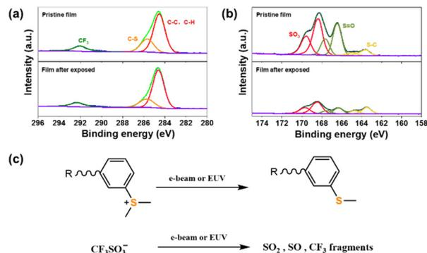
Fig. 8 (a) C 1s and (b) S 2p XPS core spectra of the SnMSF<sub>4</sub> resist films before and after e-beam exposure. (c) Proposed decomposition process of sulfonium and CF<sub>3</sub>SO<sub>3</sub><sup>-</sup> units.
