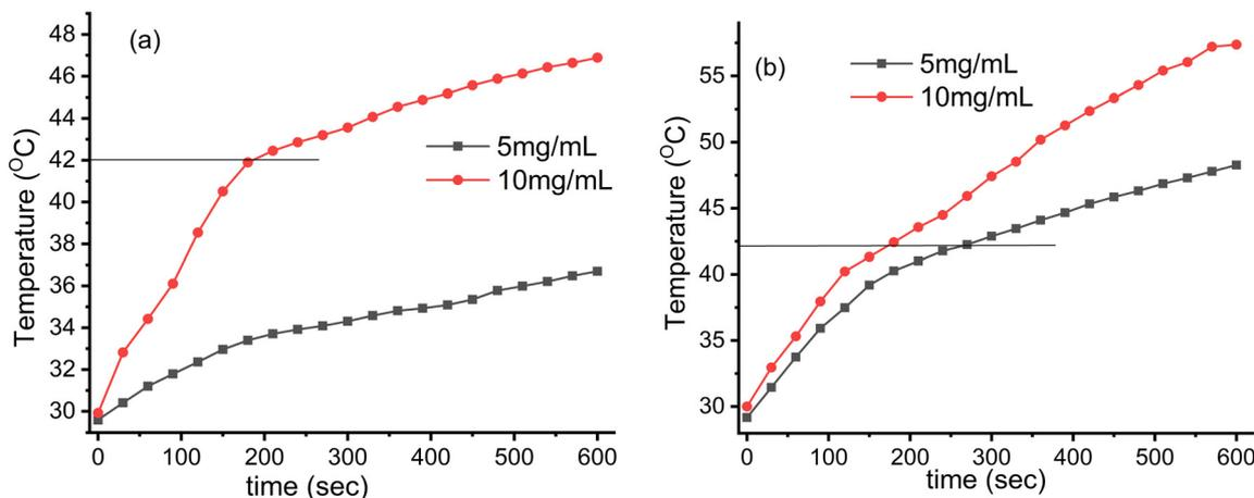
Fig. 7 Induction heating (temperature vs. time) profile of the  $\text{Fe}_3\text{O}_4@\text{SiO}_2@\text{GdPO}_4:\text{Tb}^{3+},\text{Ce}^{3+}$  nanocomposites at different concentrations and magnetic field strengths ( $H_f$ ) (a)  $3.05 \times 10^6$  ( $\text{kA m}^{-1} \text{s}^{-1}$ ) and (b)  $4.58 \times 10^6$  ( $\text{kA m}^{-1} \text{s}^{-1}$ ) maintained at a fixed applied frequency of 178 kHz.
