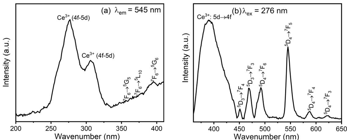
Fig. 5 (a) Excitation spectrum monitored at an emission wavelength of 545 nm and (b) emission spectrum excited at 276 nm of the CMC functionalized  $\text{Fe}_3\text{O}_4@\text{SiO}_2@\text{GdPO}_4:\text{Tb}^{3+},\text{Ce}^{3+}$  nanocomposite.
