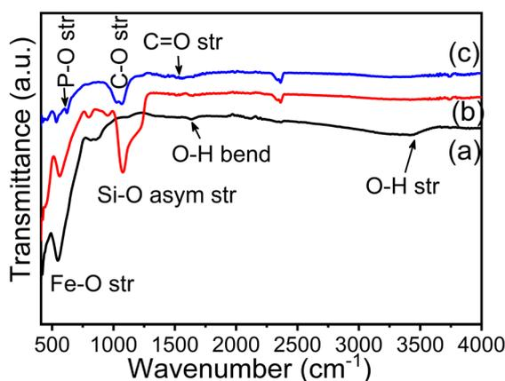
Fig. 3 FTIR spectra of (a)  $\text{Fe}_3\text{O}_4$  nanoparticles, (b)  $\text{Fe}_3\text{O}_4@ \text{SiO}_2$  nanocomposites and (c) CMC functionalized  $\text{Fe}_3\text{O}_4@ \text{SiO}_2@ \text{GdPO}_4\cdot\text{Tb}^{3+}, \text{Ce}^{3+}$  nanocomposites.
