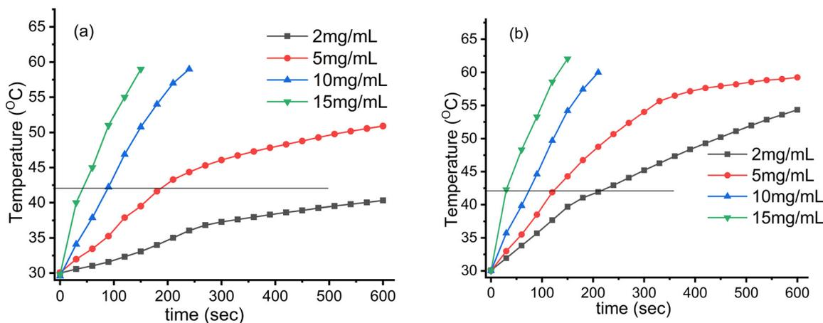
Fig. 6 Induction heating (temperature vs. time) profile of the  $\text{Fe}_3\text{O}_4$  nanoparticles at different concentrations and magnetic field strengths ( $H_f$ ) of (a)  $3.05 \times 10^6$  ( $\text{kA m}^{-1} \text{s}^{-1}$ ) and (b)  $4.58 \times 10^6$  ( $\text{kA m}^{-1} \text{s}^{-1}$ ) maintained at a fixed applied frequency of 178 kHz.
