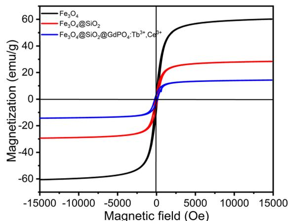
Fig. 4 Room-temperature magnetization vs. magnetic field strength for the  $\text{Fe}_3\text{O}_4$  nanoparticle,  $\text{Fe}_3\text{O}_4@ \text{SiO}_2$  nanocomposite and CMC functionalized  $\text{Fe}_3\text{O}_4@ \text{SiO}_2@ \text{GdPO}_4\cdot\text{Tb}^{3+}, \text{Ce}^{3+}$  nanocomposite.
