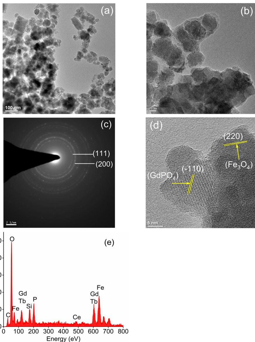
Fig. 2 TEM images of (a)  $\text{Fe}_3\text{O}_4$  nanoparticles and (b) CMC functionalized  $\text{Fe}_3\text{O}_4@SiO_2@GdPO_4:Tb^{3+},Ce^{3+}$  nanocomposites. (c) SAED pattern of  $\text{Fe}_3\text{O}_4$  nanoparticles, (d) HRTEM image and (e) EDS spectra of CMC functionalized  $\text{Fe}_3\text{O}_4@SiO_2@GdPO_4:Tb^{3+},Ce^{3+}$  nanocomposites.
