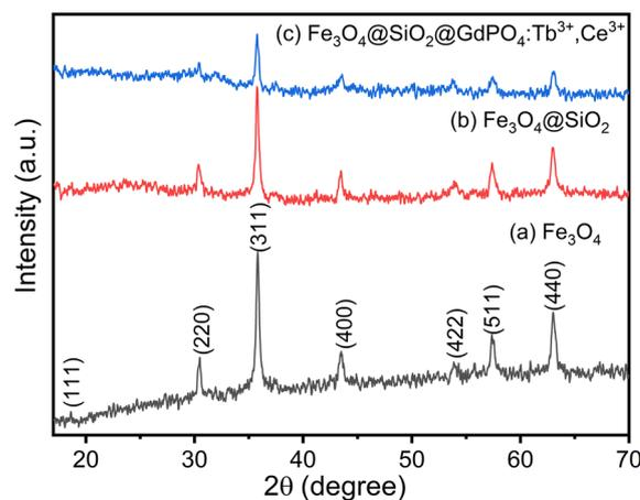
Fig. 1 XRD pattern of (a) Fe<sub>3</sub>O<sub>4</sub> nanoparticles, (b) Fe<sub>3</sub>O<sub>4</sub>@SiO<sub>2</sub> nanocomposites and (c) CMC functionalized Fe<sub>3</sub>O<sub>4</sub>@SiO<sub>2</sub>@GdPO<sub>4</sub>:Tb<sup>3+</sup>,Ce<sup>3+</sup> nanocomposites.
