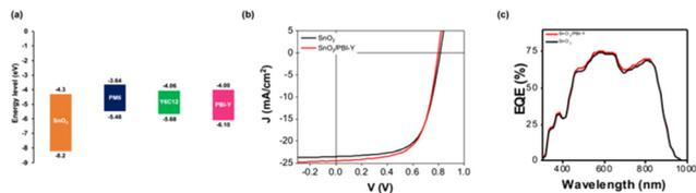
**Fig. 5** (a) The energy levels of SnO<sub>2</sub>, PM6, Y6C12 and PBI-Y. (b) *J*-*V* curves and (c) EQE spectra of spin-coated SnO<sub>2</sub>/PBI-Y devices (red) compared to reference with SnO<sub>2</sub> only (black).
