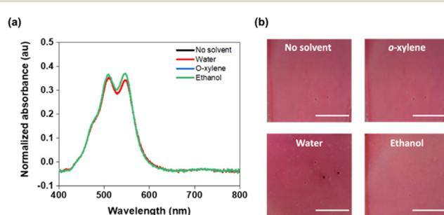
Fig. 4 (a) Optical absorption spectra and (b) photographs of 1.5 cm × 1.5 cm of glass/SnO<sub>2</sub>/PBI-Y films with no solvent and films dipped in water, *o*-xylene and ethanol for 15 seconds and then removed and left to dry. All films were spin-coated at a concentration of 0.5 mg mL<sup>-1</sup>, in air and at room temperature, onto glass substrates. The scale bar represents 1 cm.
