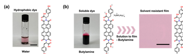
Fig. 2 Green solvent filming process. Chemical structure and photographs of PBI-Y studied in (a) water (0.5 mg mL -1 ) and (b) butylamine (0.5 mg mL -1 ) (left) and the resulting spin-coated film on plasma-cleaned glass (right). Scale bar represents 1 cm.
