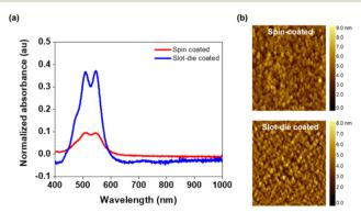
Fig. 3 (a) Absorption spectra of spin-coated and slot-die coated SnO<sub>2</sub>/PBI-Y films. (b) AFM images of spin-coated (top) and slot-die coated (bottom) SnO<sub>2</sub>/PBI-Y films. All films were cast at a concentration of 0.5 mg mL<sup>-1</sup>, in air and at room temperature.
