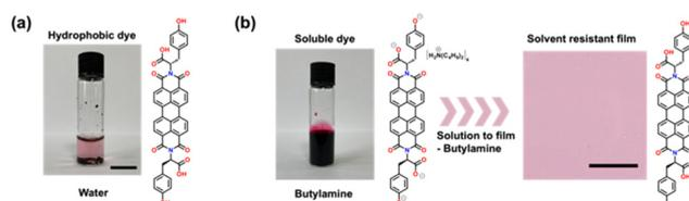
Fig. 2 Green solvent filming process. Chemical structure and photographs of **PBI-Y** studied in (a) water (0.5 mg mL<sup>-1</sup>) and (b) butylamine (0.5 mg mL<sup>-1</sup>) (left) and the resulting spin-coated film on plasma-cleaned glass (right). Scale bar represents 1 cm.
