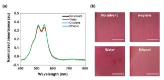
Fig. 4 (a) Optical absorption spectra and (b) photographs of 1.5 cm  $\times$ 1.5 cm of glass/SnO<sub>2</sub>/PBI-Y films with no solvent and films dipped in water, o-xylene and ethanol for 15 seconds and then removed and left to dry. All films were spin-coated at a concentration of 0.5 mg mL<sup>-1</sup>, in air and at room temperature, onto glass substrates. The scale bar represents 1 cm.
