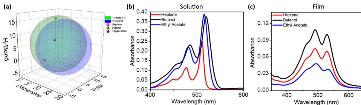
**Fig. 3** (a) The Hansen solubility spheres of F-PDIN-EH and PDIN-EH inset with heptane, butanol, and ethyl acetate HSPs. (b) Solution UV-visible absorption spectra of F-PDIN-EH in heptane, butanol, and ethyl acetate taken in a 10 mm pathlength quartz cuvette (~10<sup>-5</sup> M). (c) Thin film UV-visible absorption of F-PDIN-EH spin cast from heptane (2 mg mL<sup>-1</sup>, 1000 rpm), ethyl acetate (2 mg mL<sup>-1</sup>, 1000 rpm), and butanol (2 mg mL<sup>-1</sup>, 3000 rpm).
