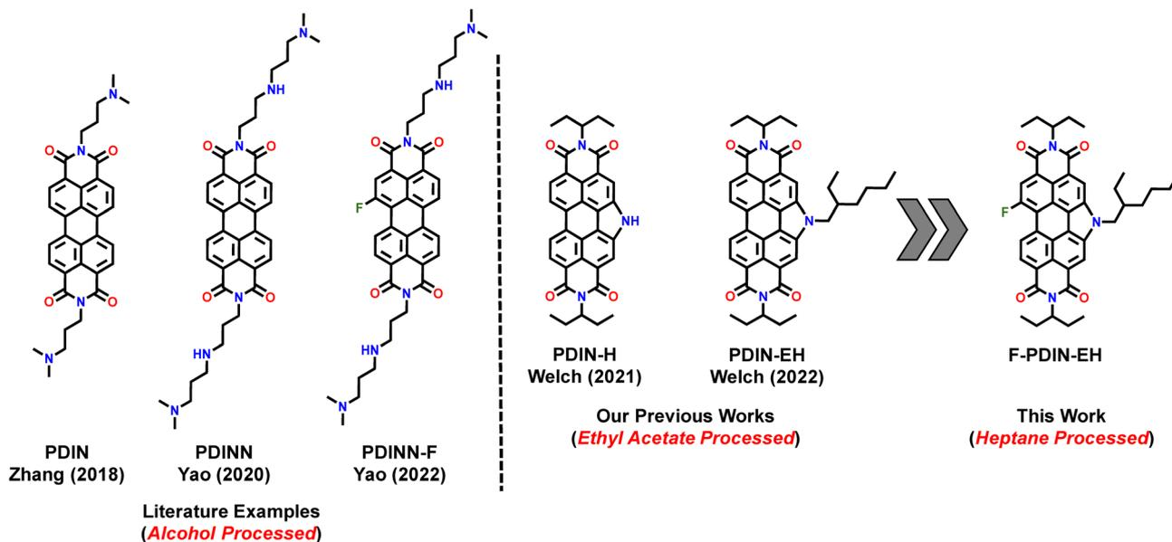
**Fig. 1** Selected PDI derived materials used as cathode interlayers in conventional organic photovoltaic devices includes PDIN,<sup>14</sup> PDINN,<sup>17</sup> PDINN-F,<sup>18</sup> PDIN-H,<sup>20</sup> and PDIN-EH<sup>21,22</sup> towards the design of the new F-PDIN-EH material.
