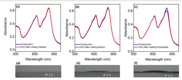
Fig. 4 The optical absorption spectra of the PM6:Y6 BHJ films before (blue) and after (red) slot-die coating (a) heptane, (b) butanol, and (c) ethyl acetate atop BHJ films. The contact angle measurements of d) heptane e) butanol, and f) ethyl acetate drops upon the BHJ.
