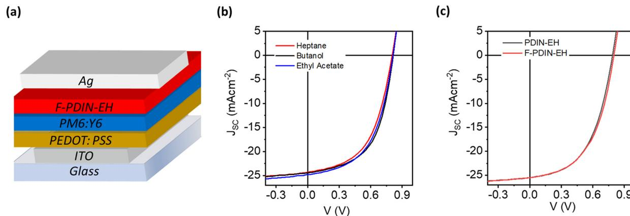
**Fig. 6** (a) Representative conventional OPV device structure hosting F-PDIN-EH as CIL. (b)  $J$ - $V$  curves of conventional OPV devices with F-PDIN-EH spin cast as a CIL. (c) Representative  $J$ - $V$  curves of conventional OPV devices with F-PDIN-EH and PDIN-EH as CIL slot-die coated from heptane.
