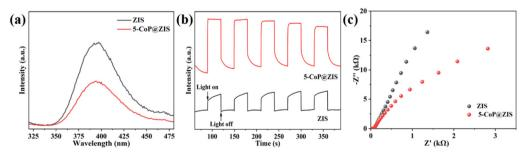
Fig. 6 (a) Steady-state PL spectra. (b) Transient photocurrent response curves. (c) EIS plots of ZIS and 5-CoP@ZIS.
