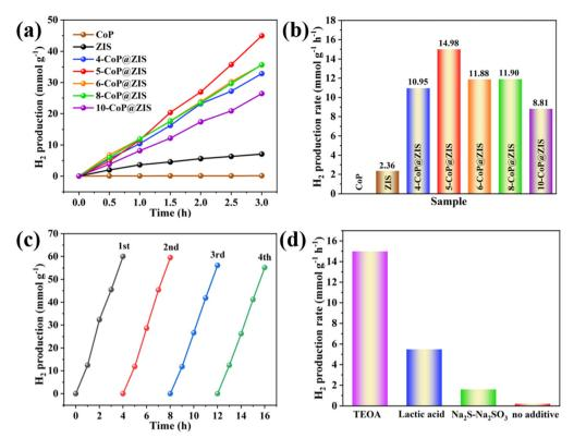
Fig. 5 Photocatalytic H<sub>2</sub> evolution performance: (a) time-yield plots of H<sub>2</sub> evolution. (b) H<sub>2</sub> evolution rate for different samples. (c) Cyclic tests of 5-CoP@ZIS. (d) Photocatalytic hydrogen evolution performance with different sacrificial reagents on 5-CoP@ZIS.
