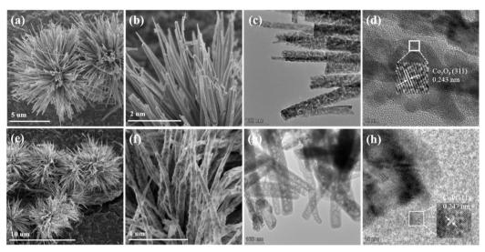
Fig. 2 SEM images of (a and b) Co<sub>3</sub>O<sub>4</sub> and (e and f) CoP. TEM images of (c) Co<sub>3</sub>O<sub>4</sub> and (q) CoP. HRTEM images of (d) Co<sub>3</sub>O<sub>4</sub> and (h) CoP.
