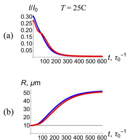
**Fig. 6** Relaxation of a waveguide formed at  $T = 25\text{ }^\circ\text{C}$  after the incident laser beam is blocked at the moment of time  $t = 2000\tau_0$  as tested by short pulses of a Gaussian beam. (a) The maximal intensity and (b) radius of the exiting probe beam (at  $z = 3\text{ mm}$ ) as functions of time. Blue- and red-colored curves correspond to the waveguides formed at light intensities of  $I_0 = 1/4I_{\text{ref}}$  and  $I_{\text{ref}}$ , respectively.
