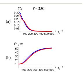
Fig. 6 Relaxation of a waveguide formed at T = 25 °C after the incident laser beam is blocked at the moment of time  $t = 2000\tau_0$  as tested by short pulses of a Gaussian beam. (a) The maximal intensity and (b) radius of the exiting probe beam (at z = 3 mm) as functions of time. Blue- and red-colored curves correspond to the waveguides formed at light intensities of  $I_0 = 1/4I_{ref}$  and  $I_{ref}$ , respectively.
