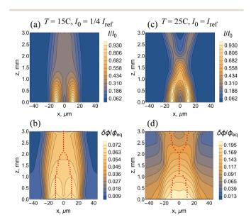
Fig. 8 Interaction between two incoherent laser beams separated by the distance of  $\Delta x = 3R_0$ . The spatial distributions of (a) intensity of light  $I/I_0$ , and (b) relative variations of the volume fraction of polymer in gel  $\delta\phi/\phi_{\rm eq}$  at T = 15 °C and  $I_0$  = 1/4 $I_{\rm ref}$ , and t = 2400 $\tau_0$ . (c) and (d): The same at T = 25 °C and  $I_0 = I_{ref}$ . In (b) and (d), the red-colored dots indicate the positions of local maxima of the intensity of light.
