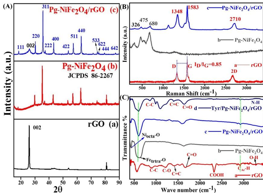
**Fig. 1** (A) XRD spectra of (a) rGO, (b) Pg-NiFe<sub>2</sub>O<sub>4</sub>, and (c) Pg-NiFe<sub>2</sub>O<sub>4</sub>/rGO nanocomposite with their respective planes. (B) Raman spectra of (a) rGO, (b) Pg-NiFe<sub>2</sub>O<sub>4</sub>, and (c) Pg-NiFe<sub>2</sub>O<sub>4</sub>/rGO nanocomposite. (C) FTIR spectra of (a) rGO, (b) Pg-NiFe<sub>2</sub>O<sub>4</sub>, (c) Pg-NiFe<sub>2</sub>O<sub>4</sub>/rGO, and (d) Tyr/Pg-NiFe<sub>2</sub>O<sub>4</sub>/rGO, in transmittance mode.
