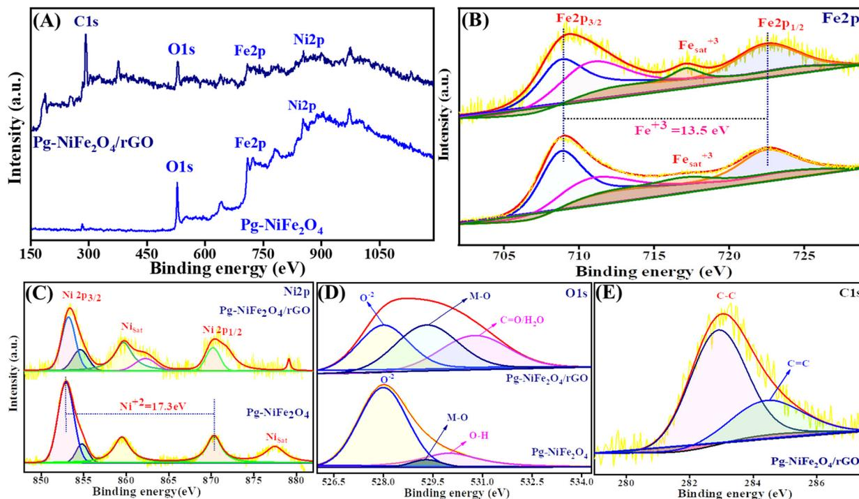
Fig. 6 XPS survey spectra of (A) Pg-NiFe<sub>2</sub>O<sub>4</sub> and Pg-NiFe<sub>2</sub>O<sub>4</sub>/rGO. (B) Fe 2p deconvoluted spectra of XPS having different binding-energy states. (C) Ni 2p deconvoluted spectra of XPS having different binding-energy states. (D and E) O 1s and C 1s deconvoluted spectra of XPS having different binding-energy states.
