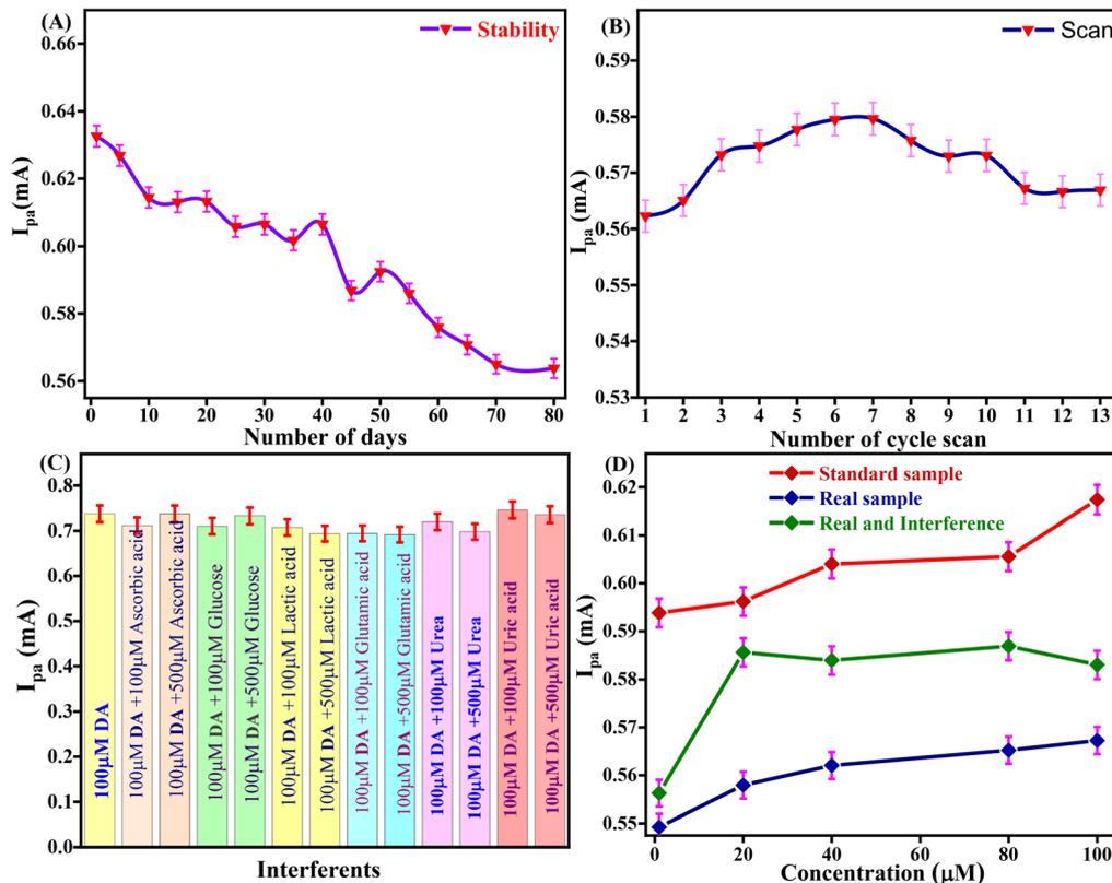
**Fig. 10** (A and B) Stability and reusability of the Tyr/Pg-NiFe<sub>2</sub>O<sub>4</sub>/rGO/ITO bioelectrode. (C) Interference study with DA. (D) Standard sample, real spiked sample, and real sample with interference being due to analytes of different concentration.
