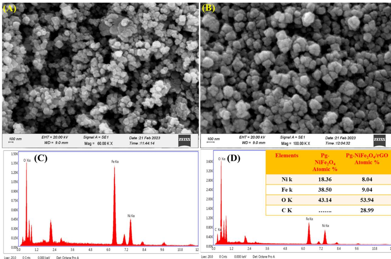
Fig. 4 SEM image of (A) Pg-NiFe<sub>2</sub>O<sub>4</sub>. (B) EDX image of Pg-NiFe<sub>2</sub>O<sub>4</sub>. (C) SEM image of Pg-NiFe<sub>2</sub>O<sub>4</sub>/rGO. (D) EDX image of Pg-NiFe<sub>2</sub>O<sub>4</sub>/rGO nanocomposite showing elemental composition (atomic%) in tabular form.
