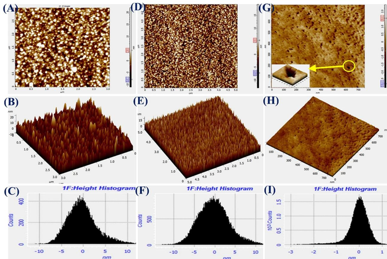
Fig. 5 A–C are AFM images denoting 2D, 3D, and the height histogram of Pg-NiFe<sub>2</sub>O<sub>4</sub>. D–F are AFM images denoting 2D, 3D, and the height histogram of Pg-NiFe<sub>2</sub>O<sub>4</sub>/rGO. G–I are AFM images denoting 2D, 3D, and the height histogram of Tyr/Pg-NiFe<sub>2</sub>O<sub>4</sub>/rGO.
