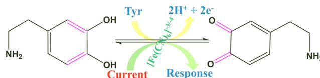
**Scheme 1** Electrochemical oxidation of DA on the surface of the Tyr/Pg-NiFe<sub>2</sub>O<sub>4</sub>/rGO/ITO bioelectrode.
