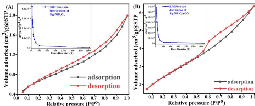
Fig. 7 A and B Specific surface area of Pg-NiFe<sub>2</sub>O<sub>4</sub> and Pg-NiFe<sub>2</sub>O<sub>4</sub>/rGO based on BET calculation. Inset image shows the pore-size distribution.
