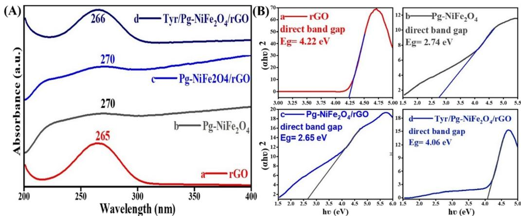
Fig. 2 (A) UV-visible absorbance spectra of (a) rGO, (b) Pg-NiFe<sub>2</sub>O<sub>4</sub>, (c) Pg-NiFe<sub>2</sub>O<sub>4</sub>/rGO, and (d) Tyr/Pg-NiFe<sub>2</sub>O<sub>4</sub>/rGO nanocomposites. (B) Band gap analysis by Tauc plots of (a) rGO, (b) Pg-NiFe<sub>2</sub>O<sub>4</sub>, (c) Pg-NiFe<sub>2</sub>O<sub>4</sub>/rGO, and (d) Tyr/Pg-NiFe<sub>2</sub>O<sub>4</sub>/rGO nanocomposites.
