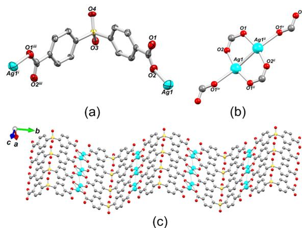
Fig. 2 Structural representations of **1**. (a) Connectivity of μ<sub>6</sub>-sdba<sup>2-</sup> ligand. (b) Coordination environment around Ag1 centers (some atoms are omitted for clarity). Symmetry code: i (–1 – x, ½ + y, 1 – z); ii (–1 – x, 1 – y, 1 – z); iii (x, ½ – y, z); iv (x, y, 1 + z); v (–1 – x, 1 – y, –z). (c) 2D metal-organic layer along the *bc* plane. Ag (cyan), O (red), S (yellow), C (gray).
