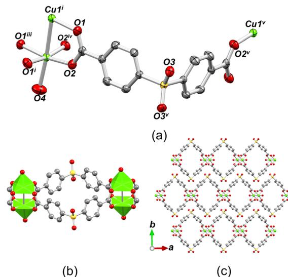
**Fig. 4** Structural representations of **2**. (a) Coordination of  $\mu_4$ -sdba<sup>2-</sup> ligand to copper centers. Symmetry codes: i (–1 – *x*, *y*, 2 – *z*); iii (1 – *x*, 1 – *y*, 2 – *z*); iv (*x*, 1 – *y*, *z*); v (–*x*, *y*, –*z*). (b) Representation of paddlewheel Cu<sub>2</sub> units. (c) 1D coordination polymer chains along the *a* axis (CCDC code: VIZRAZ).
