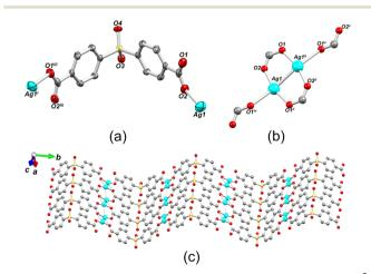
Fig. 2 Structural representations of 1. (a) Connectivity of  $\mu_6$ -sdba<sup>2-</sup> ligand. (b) Coordination environment around Ag1 centers (some atoms are omitted for clarity). Symmetry code: i  $(-1 - x, \frac{1}{2} + y, 1 - z)$ ; ii (-1 - x, 1 - z)y, 1-z); iii  $(x, \frac{1}{2}-y, z)$ ; iv (x, y, 1+z); v (-1-x, 1-y, -z). (c) 2D metalorganic layer along the bc plane. Ag (cyan), O (red), S (yellow), C (gray).
