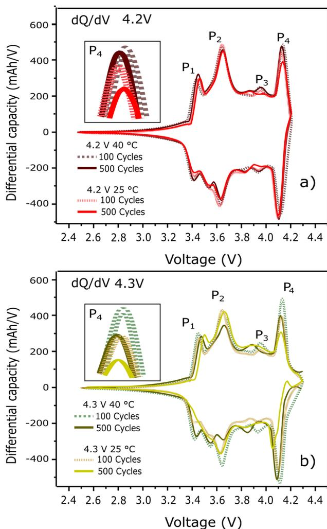
Fig. 4 dQ/dV plot after 100 and 500 cycles of the full cell at a) 4.2 V and b) 4.3 V. Traditional peak assignment: P<sub>1</sub> associated to the C<sub>6</sub> → LiC<sub>x</sub> structural changes, P<sub>2</sub> to the H1 → M transition, P<sub>3</sub> to the M → H2 transition, and P<sub>4</sub> to the H2 → H3 transition during cycling. Insets in both panels highlight the P<sub>4</sub> evolution.
