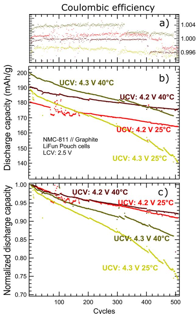
Fig. 2 a) Coulombic efficiency, b) discharge capacity, and c) normalized discharge capacity of the LiFun SC Al-surface-doped-Ni-rich/graphite pouch cells at different cycling conditions. Short periods of power outage make 4.2 V 25 °C data slightly spread around 100 cycles, but statistical trends are not altered.
