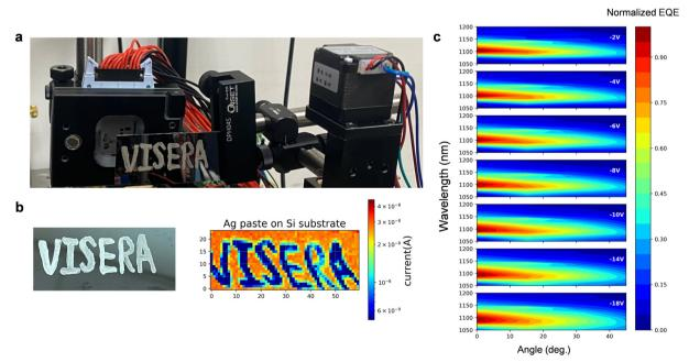
Fig. 7 a. Photo of the image scanner setup. b. Photos of the sample (Ag paste on Si substrate) for the measurement (left) and transmission image measured by narrowband OPD with 10.4 µm of a photoactive layer at 1100 nm under -10 V (right). c. Angularly and spectrally resolved EQE spectra of a narrowband photodiode with a photoactive layer thickness of 10.4 μm under various biases.
