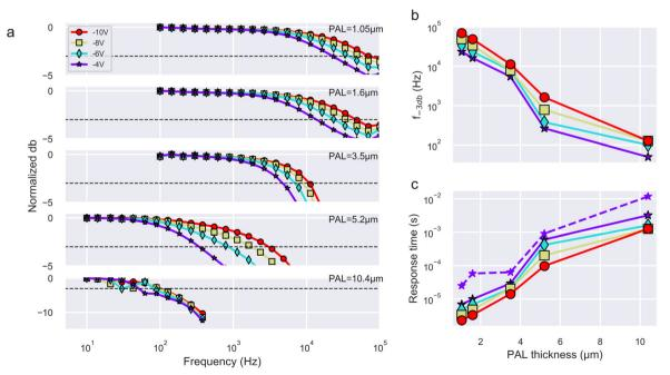
Fig. 5 a. Response time measured at various voltages for 1.05, 1.6, 3.5, 5.2, and 10.4  $\mu$ m PAL thickness; b bandwidth ( $f_{-3dB}$ ) and c. response time of the photodetector with various PAL thickness as obtained from the signal bandwidth measurements (dash line shows the response time measured by impedance fitting under a bias of -4 V).
