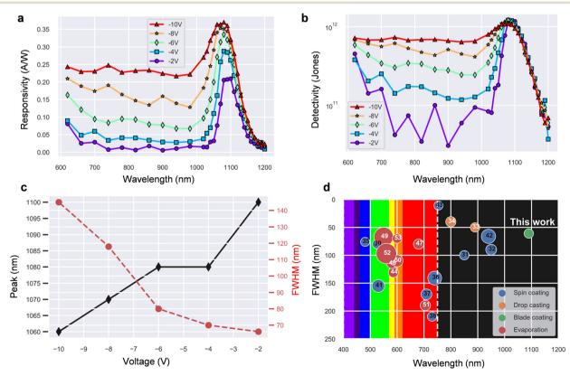
Fig. 4 a. Responsivity; b. detectivity and c. peak wavelength and corresponding FWHM at various biases. d. FWHM-wavelength plot for organic narrowband photodetector reported in the literature (the size of the circle indicates the relative detectivity value). See Table S3.†30-54
