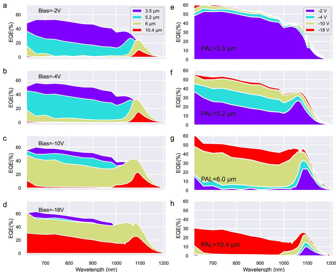
Fig. 2 a–d. EQE spectra of OPDs with various PAL thickness at the bias of  $-2$  V,  $-4$  V,  $-10$  V,  $-18$  V. e–h. EQE spectra of the OPD with PAL thickness of  $3.5$ ,  $5.2$ ,  $6.0$ ,  $10.4$   $\mu\text{m}$  at different bias voltages.
