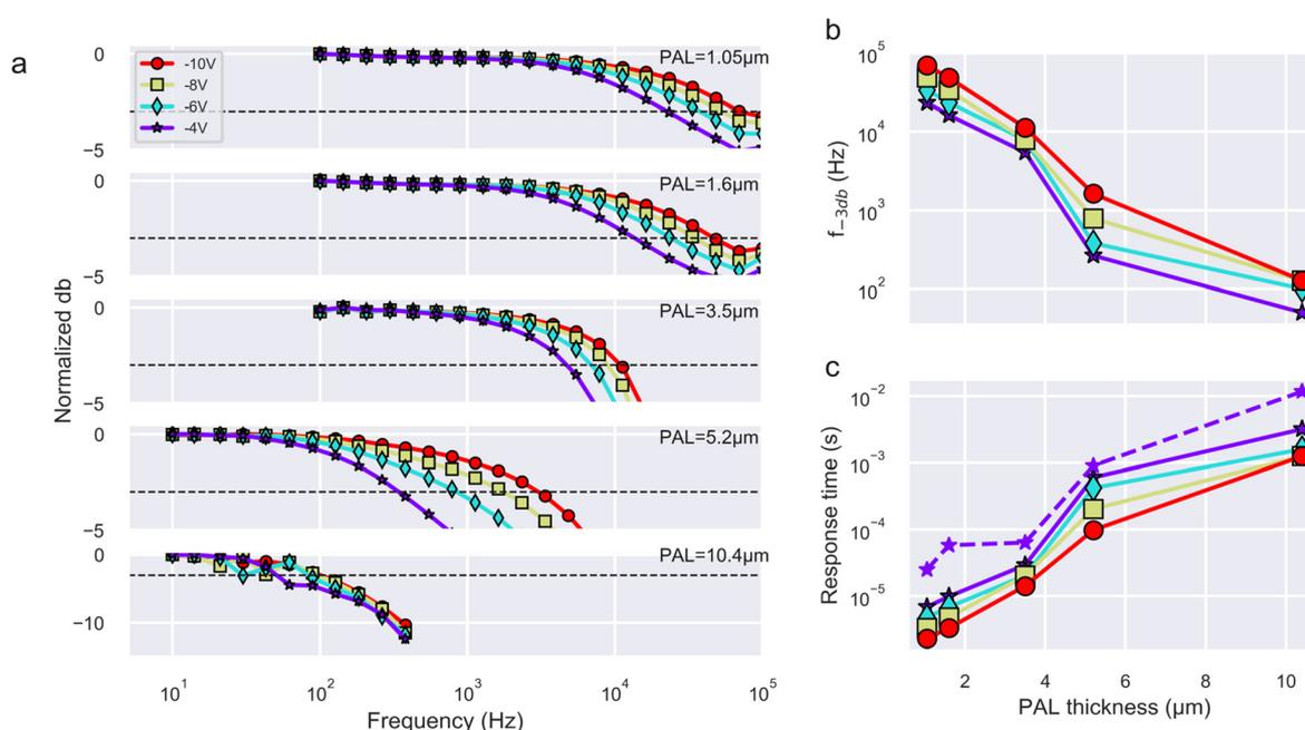
Fig. 5 a. Response time measured at various voltages for 1.05, 1.6, 3.5, 5.2, and 10.4  $\mu\text{m}$  PAL thickness; b bandwidth ( $f_{-3dB}$ ) and c. response time of the photodetector with various PAL thickness as obtained from the signal bandwidth measurements (dash line shows the response time measured by impedance fitting under a bias of -4 V).
