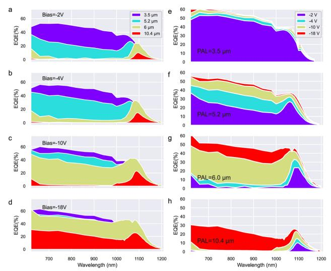
Fig. 2 a-d. EQE spectra of OPDs with various PAL thickness at the bias of -2 V, -4 V, -10 V, -18 V. e-h. EQE spectra of the OPD with PAL thickness of 3.5, 5.2, 6.0, 10.4 µm at different bias voltages.
