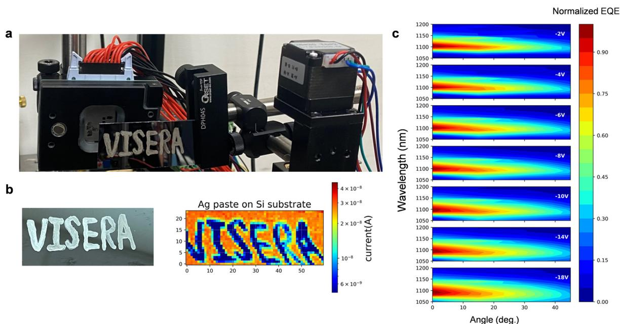
**Fig. 7** a. Photo of the image scanner setup. b. Photos of the sample (Ag paste on Si substrate) for the measurement (left) and transmission image measured by narrowband OPD with 10.4  $\mu\text{m}$  of a photoactive layer at 1100 nm under  $-10$  V (right). c. Angularly and spectrally resolved EQE spectra of a narrowband photodiode with a photoactive layer thickness of 10.4  $\mu\text{m}$  under various biases.
