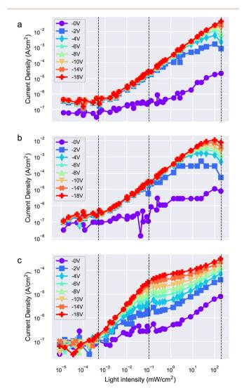
Fig. 6 Linear dynamic range of the photodetector with PAL thickness of: a. 1.05  $\mu$ m, b. 3.5  $\mu$ m, and c. 6  $\mu$ m measured at 808 nm.
