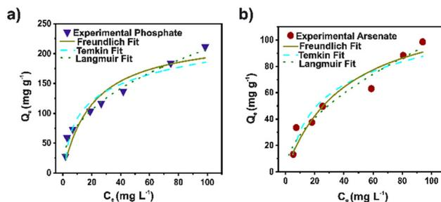
Fig. 3 Langmuir, Freundlich, and Temkin isotherm fit for a) phosphate (blue) and b) arsenate (red) using DUT-5.
