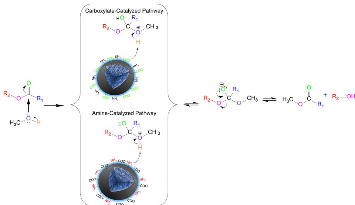
**Fig. 3** Proposed transesterification reaction mechanism using the N-CDs. Two pathways are possible for the proton abstraction from the tetrahedral intermediate, through the carboxylates or the amine groups.
