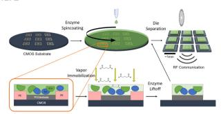
Patterned thin film enzyme electrodes via spincoating and glutaraldehyde vapor crosslinking: towards scalable fabrication of integrated sensoron-CMOS devices
