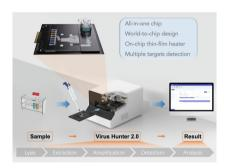
A syndromic diagnostic assay on a macrochannelto-digital microfluidic platform for automatic identification of multiple respiratory pathogens
