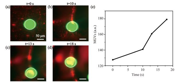
Fig. 3 Enrichment process of different sizes of fluorescent particles (1  $\mu$ m and 75  $\mu$ m). The red fluorescence corresponds to 1  $\mu$ m particles, while the green fluorescence is associated with 75  $\mu$ m particles. (a) Before applying electronic power to the IDT. (b) Formation of particle clusters after 10 s actuation, (c) 13 s actuation, and (d) 18 s actuation. (e) Mean gray values variation curves in the process of enrichment.
