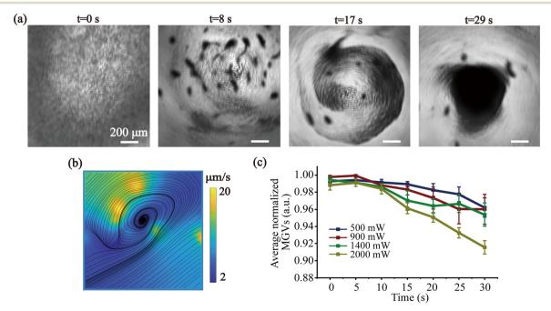
Fig. 2 (a) Concentration process of the 5 μm particles during acoustic treatment. (b) Flow velocity profile of particle concentration during acoustic treatment. (c) Analysis of the effect of input power on the particle enrichment.
