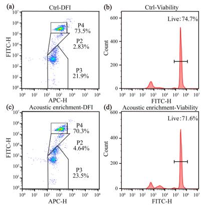
Fig. 9 The sperm DNA structure analysis post-acoustic enrichment. (a) the DFI and HDS of the control group without acoustic enrichment, (b) the sperm viability of the control group without acoustic enrichment, (c) the DFI and HDS post-acoustic enrichment, (d) the sperm viability postacoustic enrichment
