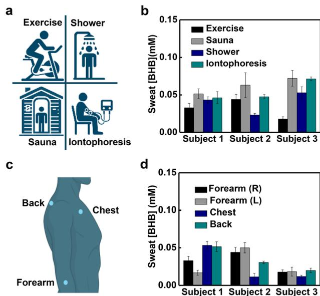
**Fig. 3** Sweat generation, collection and colorimetric analysis of [BHB] in human trials. a) Schematic illustration of four different sweat generation methods. b) Measured [BHB] in sweat generated from three subjects using various sweat generation methods. c) Schematic illustration of various locations for mounting the devices. d) Measured [BHB] in sweat generated from various body locations of three subjects during exercise.
