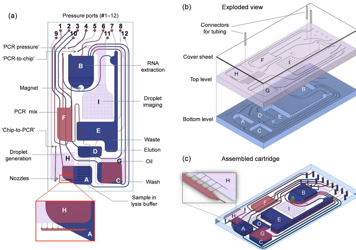
**Fig. 2** Microfluidic cartridge used for implementation of the analytical process. (a) Cartridge design (top view). Color coding is used to represent two different levels of the cartridge, with the bottom level in dark blue and the top level in light pink. The inset shows the droplet generation unit. (b) and (c) 3D renderings of the cartridge configuration revealing the microfluidic features implemented on the top and bottom levels (b) before and (c) after assembly.
