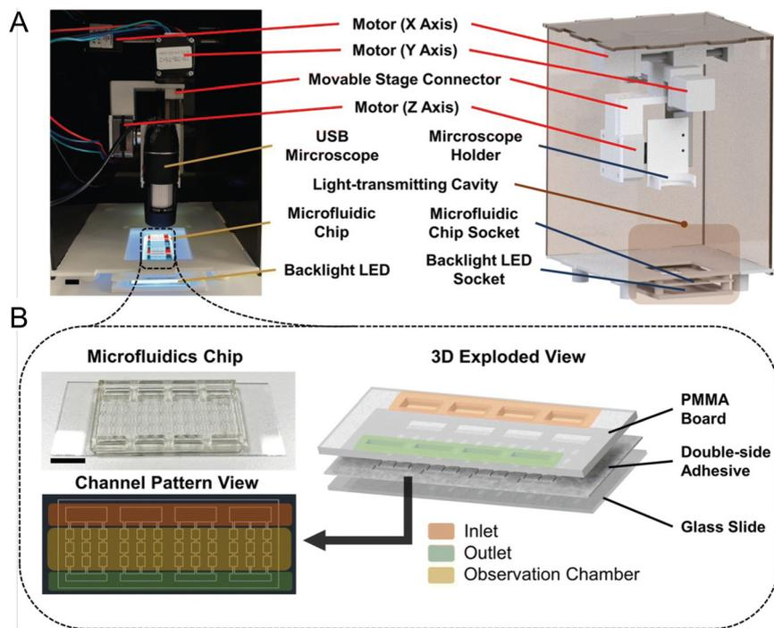
**Fig. 4** Automated and intelligent microfluidic platform (AIMP) for detecting HABs, as reported by Zheng *et al.* (A) Actual image and design schematic of the imaging part of the AIMP. (B) Schematic and image of the microfluidic chip used to load and observe microalgae (reproduced from ref. 58, CC BY 4.0, 2023).
