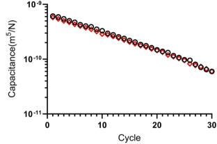
Fig. 5 Forced-air oscillator capacitance drops as the syringe fluid volume is evacuated. As the syringe pump runs, and the syringe fluid volume reduces, the total (syringe and fluid) capacitance drops over time, or as presented here after each cycle of oscillations. A) 100  $\mu m$ thick membrane and B) 20  $\mu m$  membrane oscillator system. Oscillators were run at 500 and 200  $\mu L$  min<sup>-1</sup> respectively and a 60 mL syringe.
