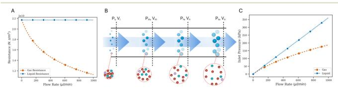
Fig. 1 (A) Comparing the resistance of a straight channel for an incompressible liquid and a compressible gas as a function of flow rate. (B) Schematic for the flow of gas through a straight channel. Density varies with pressure; therefore, the volumetric flow rate is variable while the mass flow rate is constant. (C) To drive a higher flow rate through a channel, the marginal increase in inlet pressure required for gas is lower than that for liquid.
