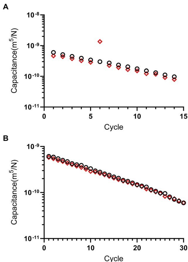
**Fig. 5** Forced-air oscillator capacitance drops as the syringe fluid volume is evacuated. As the syringe pump runs, and the syringe fluid volume reduces, the total (syringe and fluid) capacitance drops over time, or as presented here after each cycle of oscillations. A) 100  $\mu\text{m}$  thick membrane and B) 20  $\mu\text{m}$  membrane oscillator system. Oscillators were run at 500 and 200  $\mu\text{L min}^{-1}$  respectively and a 60 mL syringe.
