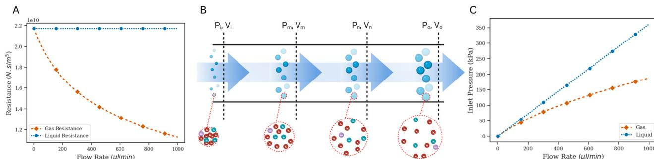
**Fig. 1** (A) Comparing the resistance of a straight channel for an incompressible liquid and a compressible gas as a function of flow rate. (B) Schematic for the flow of gas through a straight channel. Density varies with pressure; therefore, the volumetric flow rate is variable while the mass flow rate is constant. (C) To drive a higher flow rate through a channel, the marginal increase in inlet pressure required for gas is lower than that for liquid.
