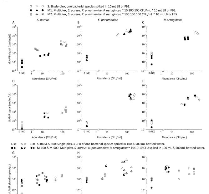
Fig. 6 The dLAMP results from multiplex (S. aureus, K. pneumoniae, and P. aeruginosa) samples in various matrices: A-C) LB, D-F) FBS, and G-I) bottled water.
