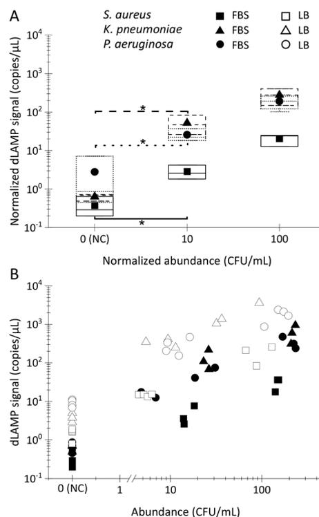
**Fig. 4** The dLAMP detection results of low-abundance bacteria in a complex background (FBS). A) Normalized dLAMP signals for normalized abundances of FBS samples, Welch's *t*-test to evaluate the detection performance (\*: *p*-value < 0.05). B) The scatter plot of dLAMP signal along with the experimentally counted abundances via plating-counting, for LB and FBS spiked samples.
