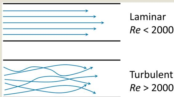
Box Fig. 1. Laminar flow and turbulent flow. The velocity profiles are portrayed in blue lines and the black lines represent channel walls.
