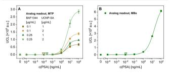
Fig. 3 Calibration curves of the (A) MTP- and (B) MB-based ULISA for PSA detection in 50% serum. The empty triangles represent the LODs, the error bars represent the standard deviations of three wells.
