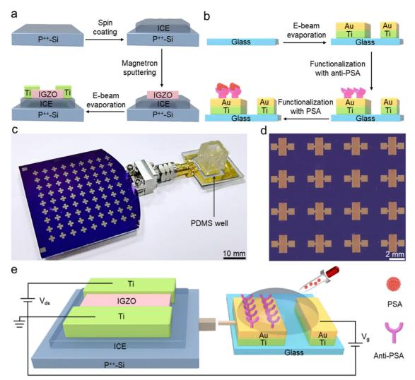
Fig. 1 Construction of IGZO transistor-based biosensor for PSA detection. Schematic illustration of fabrication process of (a) electrolyte-gated IGZO transistor and (b) extended sensing pad. (c) Optical image of electrolyte-gated IGZO transistor and extended sensing pad. (d) Microscope image of 4 × 4 IGZO transistor array. (e) Schematic diagram illustrating working mechanism and circuit connection of IGZO transistor-based biosensor.
