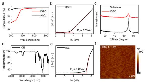
Fig. 2 Fundamental characterization of the IGZO and ICE thin film. (a) UV-visible transmittance of the sapphire ( $Al_2O_3$ ) and IGZO film. (b) Fitted  $E_a$ of the IGZO film. (c) XRD of the Si substrate and the IGZO film. (d) Fitted  $E_{\rm gr}$  (e) FTIR spectrum, and (f) AFM image of the ICE film.
