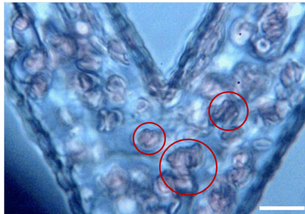
Fig. 5 Aggregated RBCs with hematocrit of ten in the presence of dextran ( H_{\text{dex}} = 10 ) at the apex of the bifurcation, imaged using a 100 \times air objective. The red circles indicate examples of clusters; the scale bar represents 15 \mu\text{m} .
