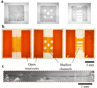
Fig. 4 Shallow channels with sacrificial films. a) Pictures of the xurographed soluble films before integration. b) Pictures of red dye in the chips after film integration and solubilisation. c) SEM image of the chip in b-left, cut in half following the red line on b.
