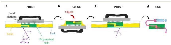
Fig. 1 Concept illustration of the print-pause-print strategy. a) Printing of a first part (pre-pause part). b) Pausing, removal of the building platform, removal of resin excess and positioning of the object to integrate. c) Resuming of the print (post-pause part). d) Cleaning and developing of the detached chip.
