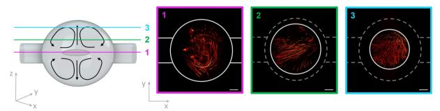
Fig. 5 Acoustic streaming in the spherical microchamber. A sketch of the spherical microchamber with acoustic streaming is shown on the left side. The recorded layers 1–3 in xy-direction are marked in different colours. On the right side, the acoustic streaming of 1  $\mu$ m microparticles is demonstrated for each layer in the SMC. Scale bar: 100  $\mu$ m.
