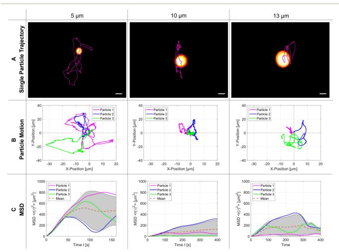
Fig. 4 Motion of trapped particles. A) Particle trajectory for a single PS microparticle of diameter 5 μm, 10 μm, and 13 μm – scale bar: 5 μm. Three repetitions of the particle trajectories for each diameter are presented in B). In C), we demonstrate the calculated mean square displacement of the particles over time, respectively.
