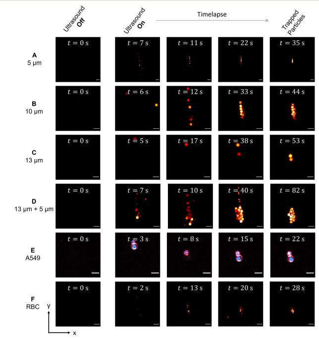
Fig. 3 Acoustic particle trapping under the two-photon-excited fluorescence microscope. From A-D different particle sizes ranging from A) 5  $\mu$ m, B) 10  $\mu$ m, C) 13  $\mu$ m and a mixture of D) 13  $\mu$ m and 5  $\mu$ m are displayed, in E) the time series of A549 cells and in F) of RBC cells are shown. Scale bar: 20  $\mu$ m.
