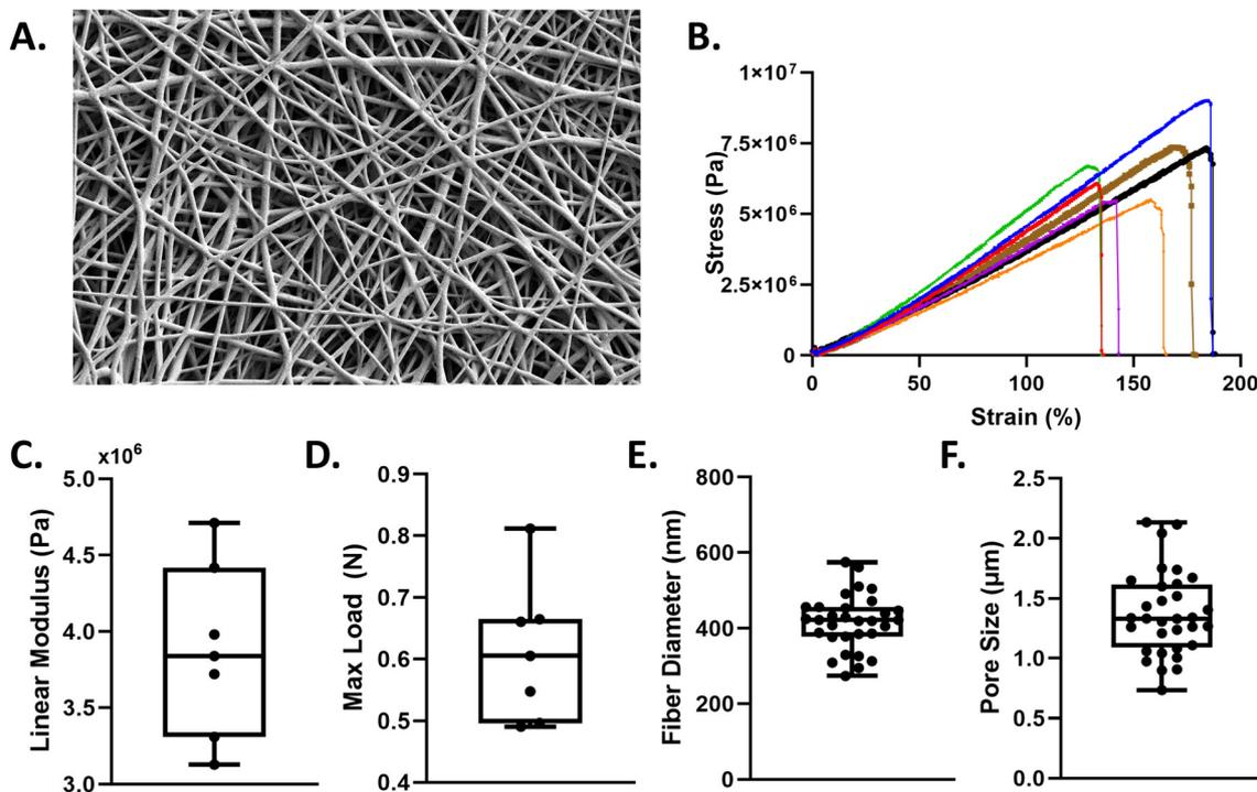
Fig. 2 Nanofiber membrane fabrication and characterization. A. SEM image of 5 wt/vol% polyurethane membrane. Scale bar = 10  $\mu\text{m}$ . B. Uniaxial tensile testing of  $n = 7$  polyurethane scaffolds illustrating the stress-strain curves. Quantification of the C. linear modulus and D. maximum load. ImageJ was used to quantify E. fiber diameter and F. pore size. Min to max all points shown.
