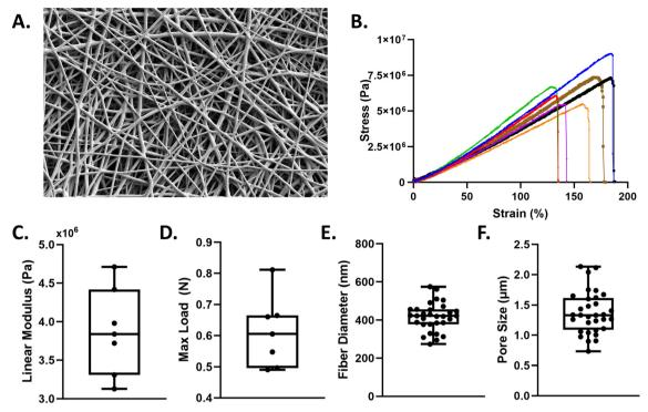
Fig. 2 Nanofiber membrane fabrication and characterization. A. SEM image of 5 wt/vol% polyurethane membrane. Scale bar = 10 μm. B. Uniaxial tensile testing of n = 7 polyurethane scaffolds illustrating the stress-strain curves. Quantification of the C. linear modulus and D. maximum load. ImageJ was used to quantify E. fiber diameter and F. pore size. Min to max all points shown.
