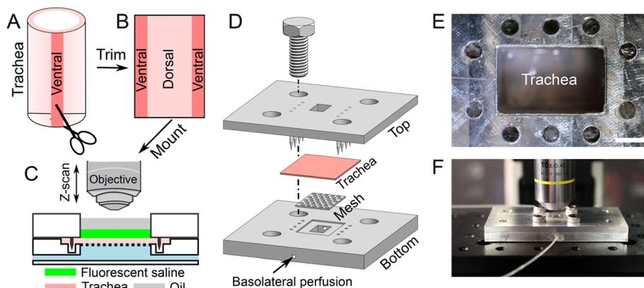
**Fig. 1** The *ex vivo* trachea-chip device to measure ASL secretion/absorption is demonstrated schematically. (A–C) Procedures to dissect tracheal tissue and mount it in the device to study ASL volume. (D) 3D drawing of the *ex vivo* trachea-chip device comprised of a top plate, a tracheal explant, a metal mesh, and a bottom plate with perfusion ports. (E and F) Photos of assembled *ex vivo* trachea-chip device on a confocal microscope stage. Scale bar is 2 mm.
