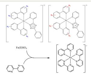
Scheme 1 (Top) Isotopically labelled ruthenium( $\shortparallel$ ) complexes used for Raman imaging of mixing of solvent streams, and (bottom) reaction between the colourless 2,2'-bipyridine and iron( $\shortparallel$ ) sulphate, to produce the red-coloured [Fe(bpy)<sub>3</sub>]<sup>2+</sup>. See Fig. S3–S6† for reference Raman spectra of compounds.
