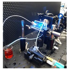
Fig. 3 Quartz chip during operando analysis of the chemical reaction described in Scheme 1 with the line-focused 473 nm laser.
