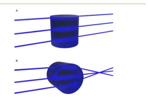
Scheme 3 Ray-diagram through (A) the non-curved and (B) curved axes of a cylindrical lens. The beam is focused and subsequently diverges along one axis only.
