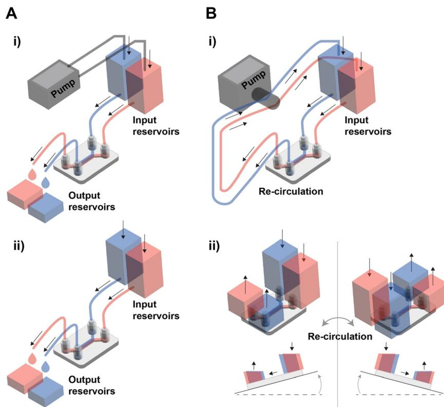
**Fig. 2** Types of fluid flow in tissue barrier chips. (A) Schematic image of open flow circuit operated by i) external pump and ii) hydrostatic pressure difference. (B) Schematic image of closed flow circuit operated by i) external pump and ii) hydrostatic pressure differences made by external tilting equipment.
