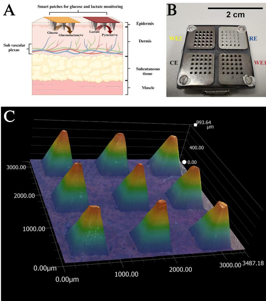
**Fig. 1** (A) Showing microanatomy of skin (created with BioRender, license number PY26AQ25FL). (B) Photograph of a patch used for physiological monitoring. (C) Images obtained using a Keyence high resolution microscope showing the morphology of the patch (each MN is 1 mm in height, 0.6 mm base, the pitch distance between the tips is 0.6 mm).
