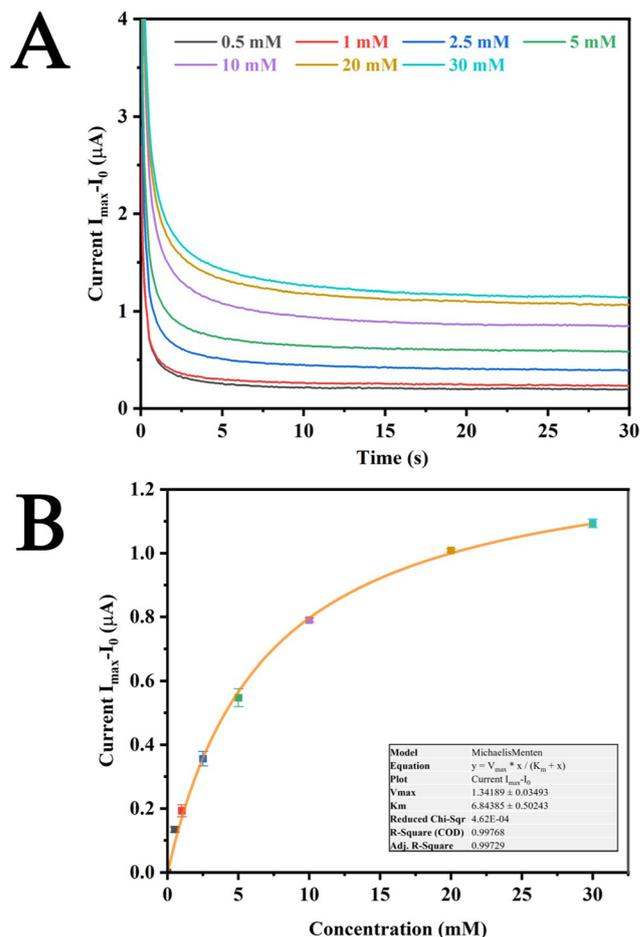
Fig. 2 *In vitro* studies: (A) chronoamperometric data obtained at a potential of 0.7 V for GOx modified Pt SPEs showing increase in baseline corrected currents and (B) dose response curves obtained for Pt SPEs from 0.5 mM to 30 mM additions of glucose (in 0.1 M PBS pH 7.4).
