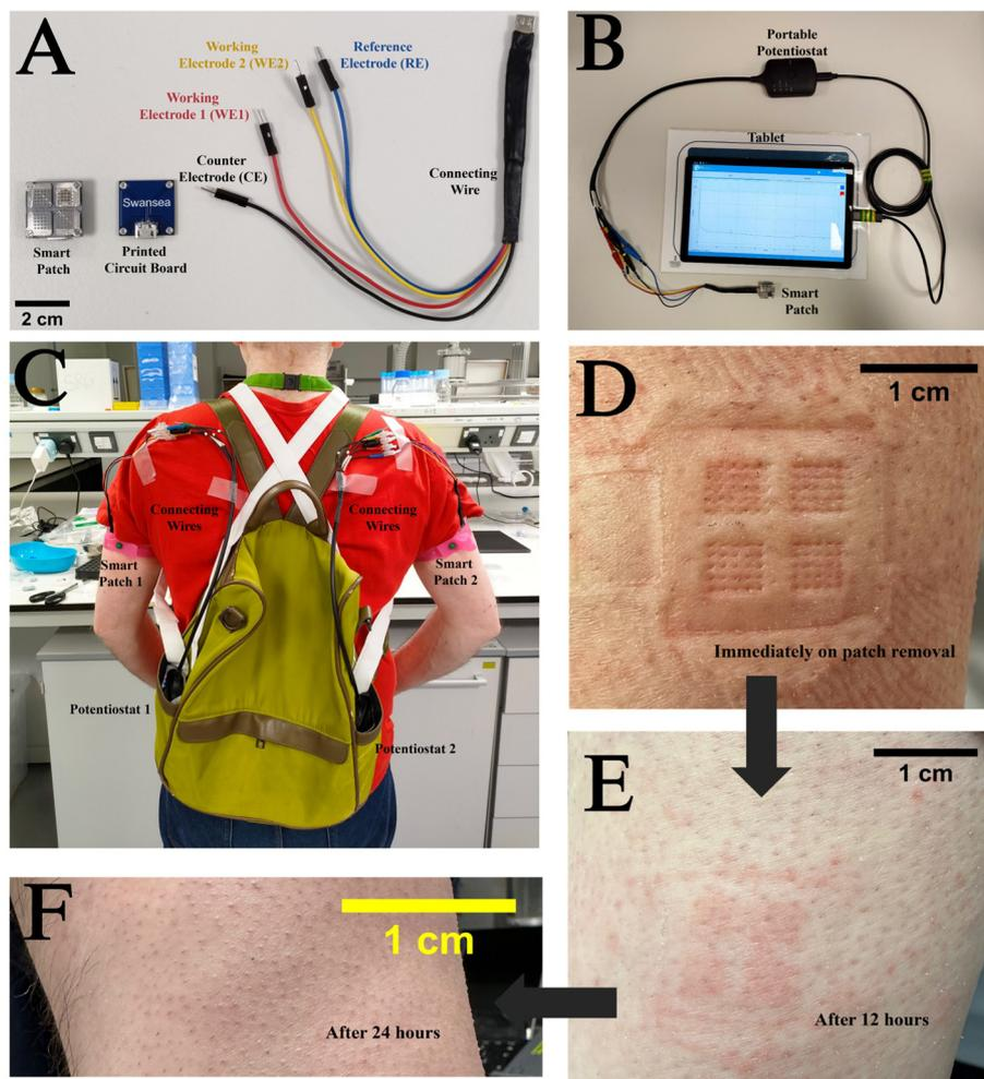
**Fig. 3** Setup for *in vivo* studies: (A) shows a metallised patch, a PCB on which it is assembled and wired with mini-USB connector. (B) Shows a commercially available portable potentiostat and a tablet to observe patch response. (C) Participant wearing a MN on the forearms for physiological monitoring. Marks on the skin (D) immediately after removal of the patches, (E) 12 hours after patch removal, and (F) 24 hours after patch removal.
