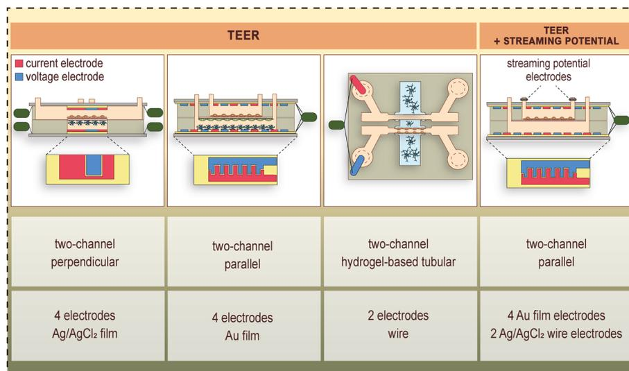
**Fig. 3** Examples of electrode placement, and measurement of TEER as well as combined TEER and streaming potential in BBB-on-chip devices.<sup>2,4,31,34</sup> Current electrodes are shown in red, whereas voltage electrodes are shown in blue color.
