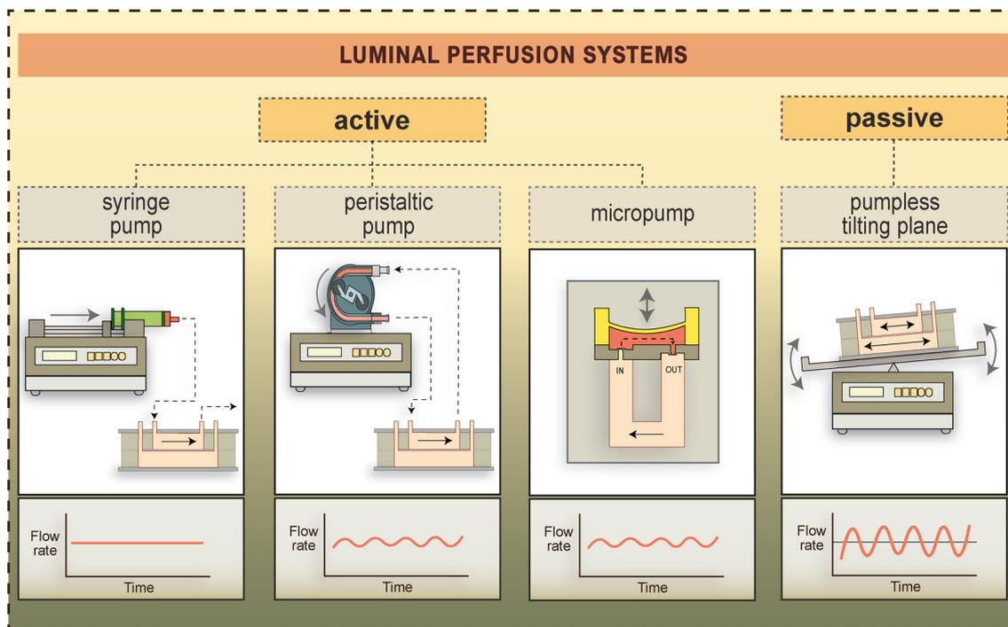
Fig. 5 Types of active and pump-free luminal perfusion systems used to generate fluid flow-induced shear stress in BBB-on-chip devices.<sup>4,24,41,101</sup> Flow rates generated by these methods over time are schematically shown in the lower panels.
