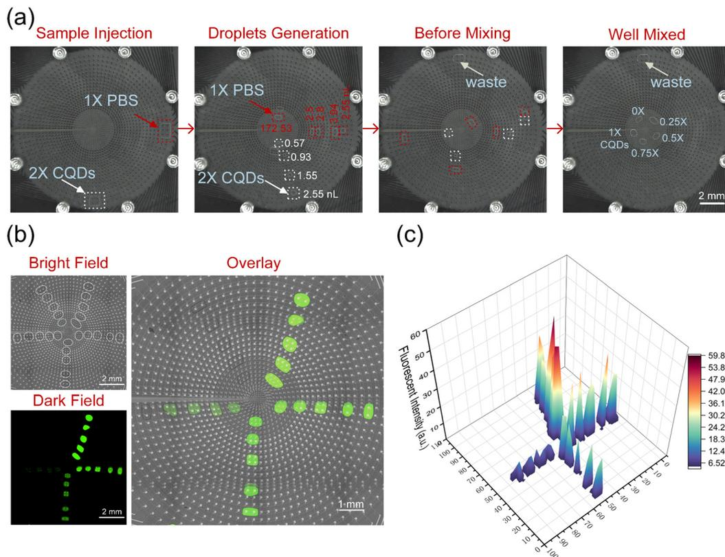
**Fig. 4** Gradient of droplet fluorescence: (a) four screenshots from Video S4† illustrate the mixing of deionized water and CQDs solution with different volumes on the AM-EWOD chip. (b) Bright-field, dark-field, and overlay images of fluorescent solutions with varying concentrations. (c) 3D stereogram of fluorescence for solutions with different concentrations.
