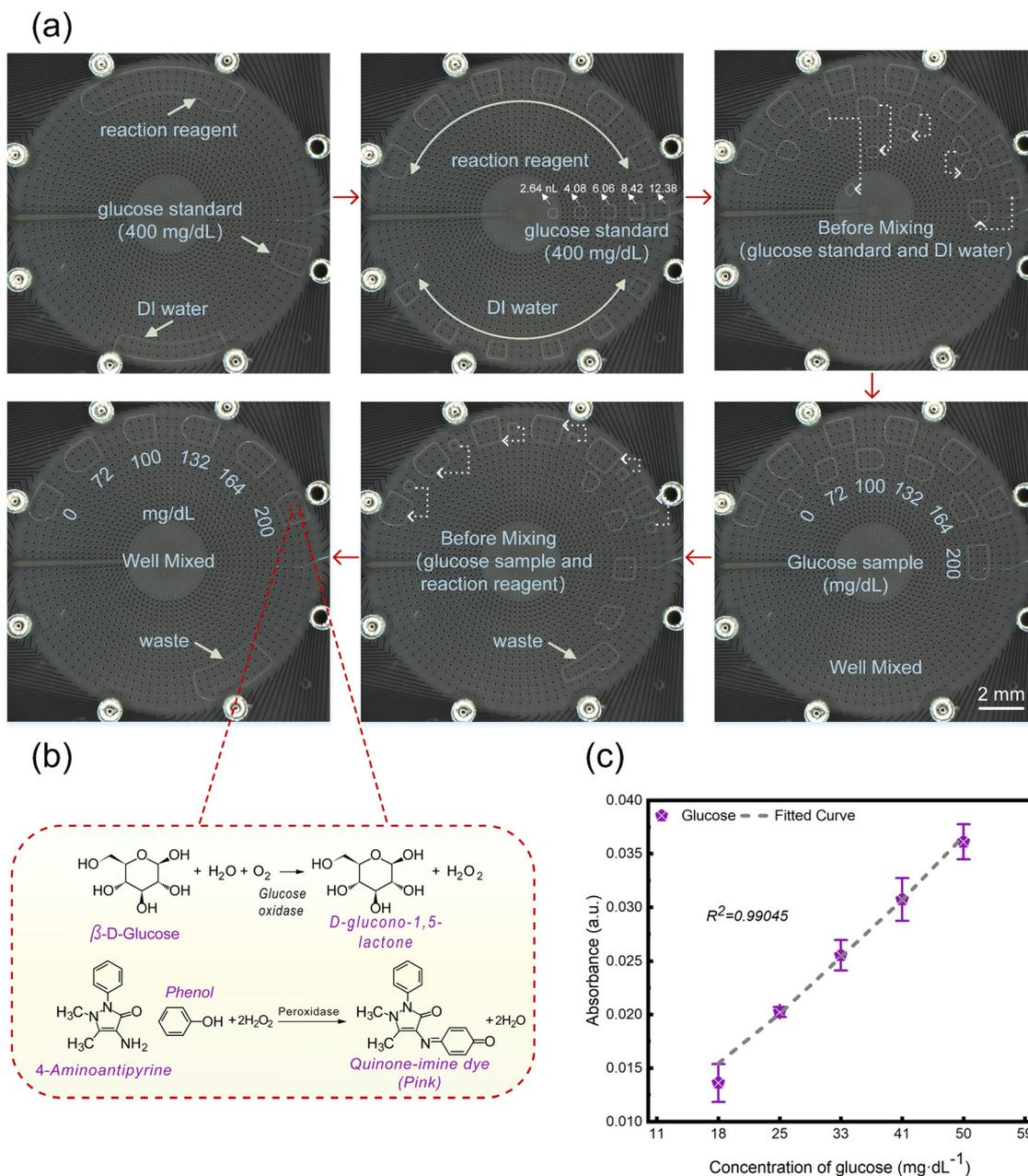
**Fig. 6** Glucose concentration experiments: (a) screenshot pictures of the glucose reaction workflow. (b) Schematic illustration of the principle of the glucose reaction. (c). Graph illustrating the relationship between different concentrations of glucose solution and absorbance.
