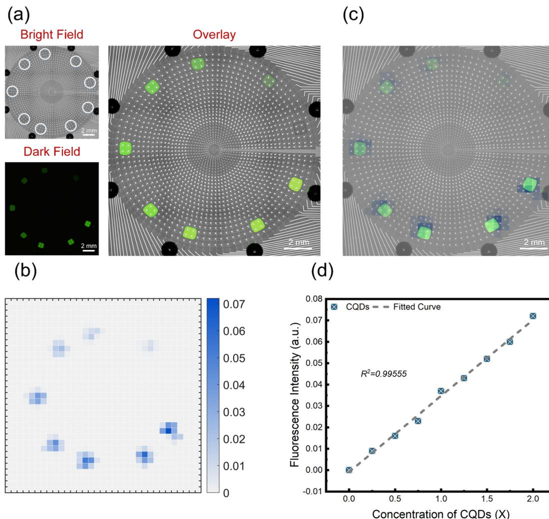
**Fig. 5** Quantitative fluorescence analysis experiments: (a) bright-field, dark-field, and overlay images of fluorescent solutions with varying concentrations. (b) Heatmap of fluorescent solutions with different concentrations. (c) Overlay images of bright-field, dark-field, and heatmap for solutions with different concentrations. (d) Graph depicting the relationship between fluorescence intensity and concentration of fluorescent solutions.
