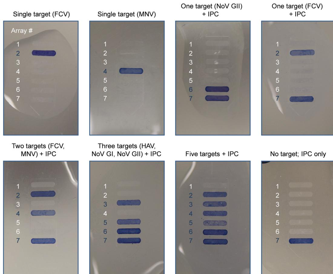
**Fig. 3** Photographs of representative Zeonor micropillar array substrates used in colorimetric virus detection assays performed off-chip by passive incubation. The configuration of the micropillar array is as follows: (#1) empty; (#2) FCV2; (#3) HAV1; (#4) MNV; (#5) NoV GI; (#6) COG2-v2; and (#7) IPC. Amplicons were produced in tubes using benchtop PCR.
