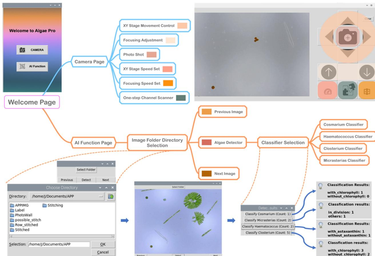
Fig. 4 Schematic illustration of the Raspberry Pi App for the AIMP and screenshots on each node.
