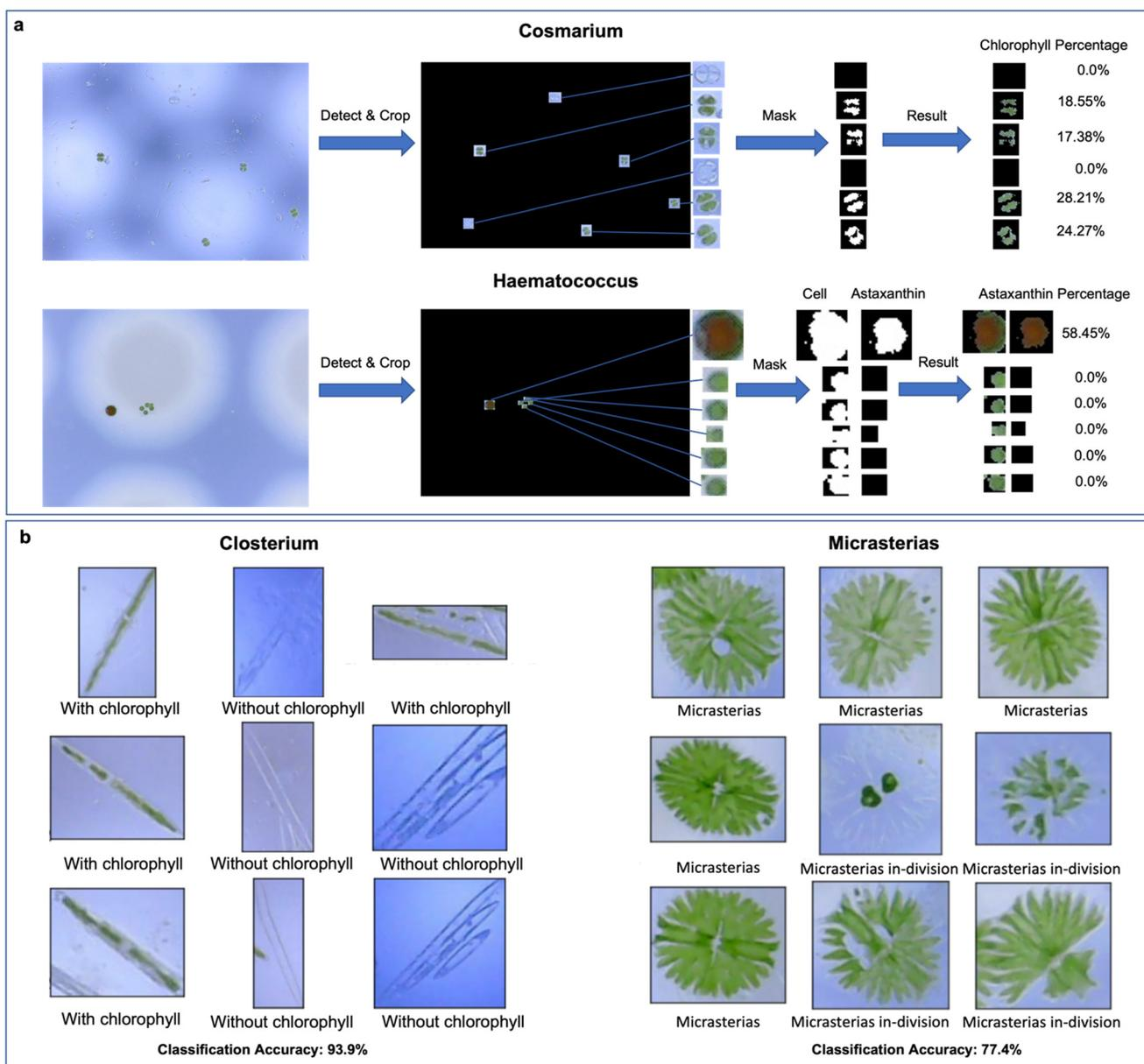
Fig. 3 Additional functions of the AIMP for monitoring the growth stage of microalgae. a) Further classification of *Cosmarium* and *Haematococcus Pluvialis* detected by the microalgae detection model by a colour extraction function. b) Further classification of *Closterium* and *Micrasterias* using two specific trained classifiers based on the EfficientNet-Lite0 architecture.
