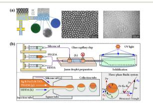
Fig. 3 Single emulsion-templated microparticles with homogeneous structures or heterogeneous structures. (a) Microfluidics device for single emulsion-templated microparticles with a homogeneous structure. Reprinted with permission from ref. 119. Copyright 2023, American Chemical Society. (b) Microfluidics device with a  $\theta$ -shaped injection tube for single emulsion-templated microparticles with heterogeneous structures. Reprinted with permission from ref. 120. Copyright 2023, Elsevier B.V.
