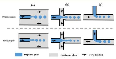
Fig. 1 Schematic of microfluidic droplet generators with dripping and jetting regimes (not to scale). (a) Co-flow, (b) flow-focusing, and (c) T-junction. Modified with permission from ref. 63. Copyright 2013, IOP Publishing Ltd. Printed in the UK and USA.
