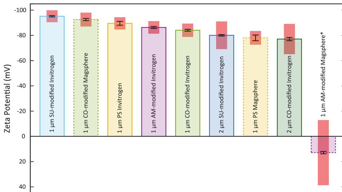
**Fig. 3** Zeta potentials for beads suspended in 10 mM HEPES determined with the Zetasizer Ultra. The mean zeta potential, standard deviation (black error bars) and the zeta potential deviation (red boxes) are shown for each sample ( $n = 5$ ). The red boxes correspond to the zeta potential deviation (\*: all particle suspension concentrations are at  $10^8$  particles per ml except the 1  $\mu\text{m}$  AM-modified particles from Magsphere which is at  $3 \times 10^9$  particles per ml).
