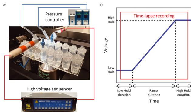
**Fig. 2** a) Experimental setup with the microfluidic chip and electrodes mounted on an inverted microscope. Reservoirs are pressurized through the modified caps by a pressure controller, and a custom voltage profile is applied by the high voltage sequencer through high voltage cables connected to the platinum electrodes. b) The voltage profile applied to the platinum electrodes with the time-lapse recording window in red.
