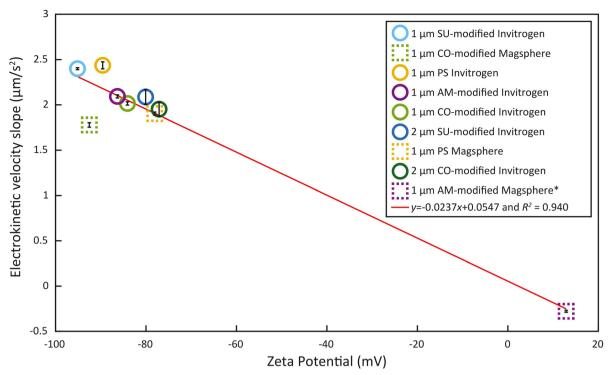
Fig. 5 Particle electrokinetic velocity slopes of 1  $\mu$ m and 2  $\mu$ m polystyrene beads with different surface functionalizations, measured by microfluidic electrokinetic characterization, as a function of  $\zeta$  (Zetasizer Ultra). PS: polystyrene, SU: sulfate, CO: carboxylate, AM: amine. Red line: data fitting.
