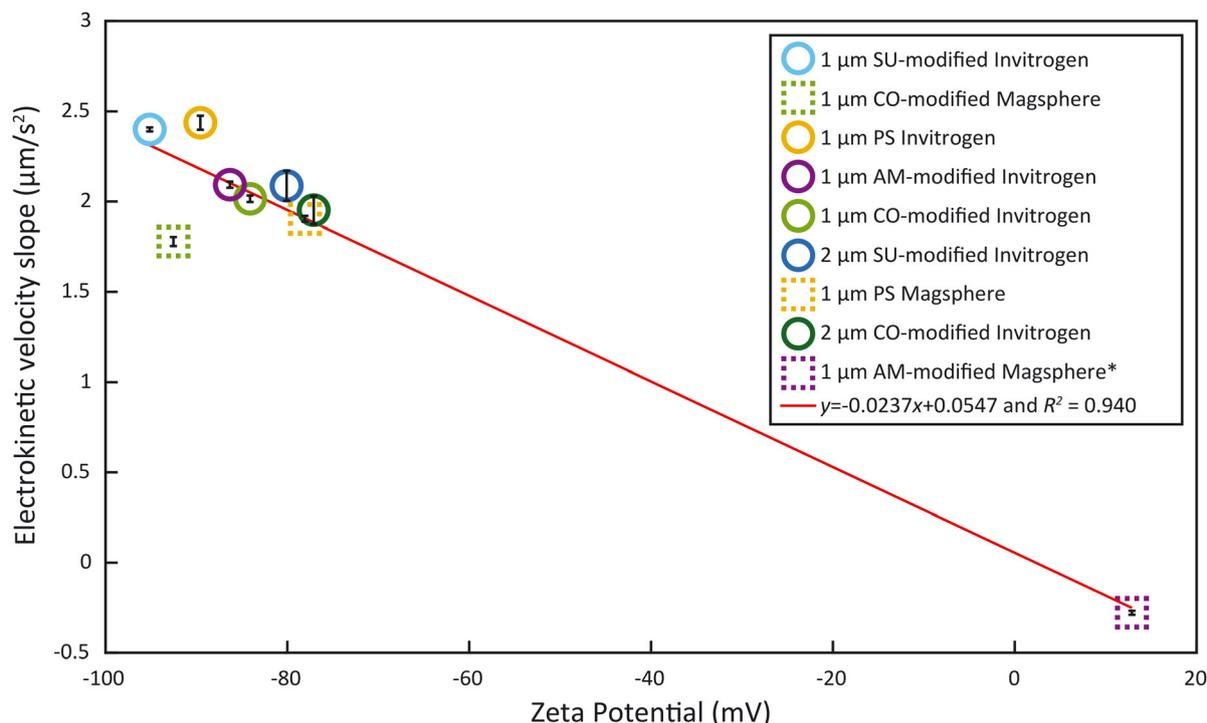
Fig. 5 Particle electrokinetic velocity slopes of 1  $\mu\text{m}$  and 2  $\mu\text{m}$  polystyrene beads with different surface functionalizations, measured by microfluidic electrokinetic characterization, as a function of  $\zeta$  (Zetasizer Ultra). PS: polystyrene, SU: sulfate, CO: carboxylate, AM: amine. Red line: data fitting.
