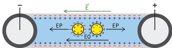
**Fig. 1** Schematic of a microchannel for particle tracking velocimetry (PTV) where charged particles are affected by two forces: electroosmosis (EO) and electrophoresis (EP) when exposed to an electric field. Counter ion charges are represented in blue and surface charges in red.
