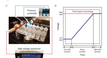
Fig. 2 a) Experimental setup with the microfluidic chip and electrodes mounted on an inverted microscope. Reservoirs are pressurized through the modified caps by a pressure controller, and a custom voltage profile is applied by the high voltage sequencer through high voltage cables connected to the platinum electrodes. b) The voltage profile applied to the platinum electrodes with the time-lapse recording window in red.
