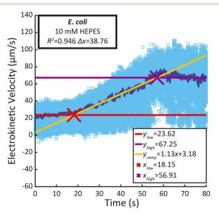
Fig. 6 Representative PTV measurements in the 100  $\mu m \times$  100  $\mu m \times$ 18 mm PMMA microchannels for E. coli MG1655 suspended in 10 mM HEPES (pH 7.2) at OD = 0.2. Light blue square: individual velocity, dark blue line: median velocity per frame.
