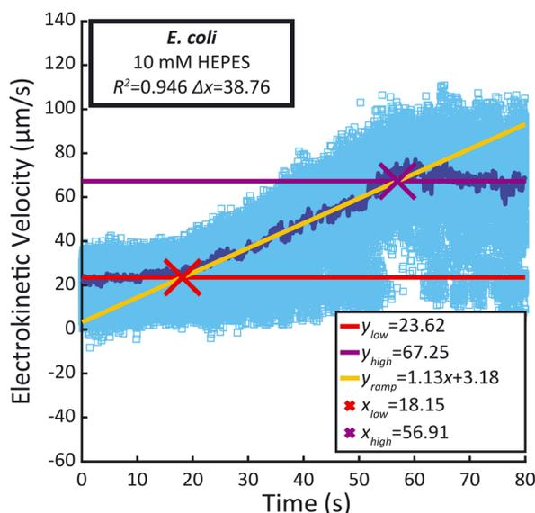
Fig. 6 Representative PTV measurements in the  $100 \mu\text{m} \times 100 \mu\text{m} \times 18 \text{ mm}$  PMMA microchannels for *E. coli* MG1655 suspended in 10 mM HEPES (pH 7.2) at OD = 0.2. Light blue square: individual velocity, dark blue line: median velocity per frame.
