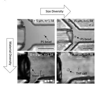
Fig. 5 Trapping versatility of OHT. Optical image of a single (a) 5  $\mu$ m polystyrene particle, (b) 15  $\mu$ m polystyrene particle, (c) 5  $\mu$ m yeast cell, and (d) 30  $\mu$ m THP cell trapped in the OHT.
