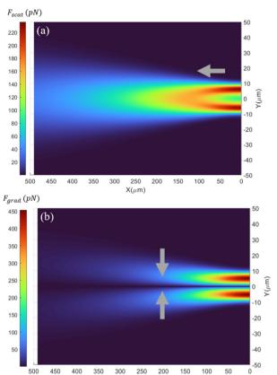
Fig. 2 Spatial distribution of (a) the optical scattering force and (b) the gradient force exerted by the laser beam from an optical fiber on a 15 μm polystyrene particle flowing in the microfluidic channel. The centre of the core of the fiber (core diameter: 6.4  $\mu$ m,  $\lambda_{laser}$  = 973 nm, P = 550 mW) is placed at the origin facing towards the positive X-axis. The magnitudes of the forces are represented in absolute values and the directions of the forces are illustrated as arrows.
