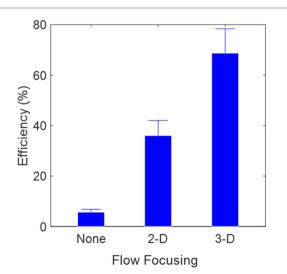
Fig. 3 Comparison of trapping efficiencies with and without 3D flow focusing.
