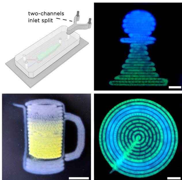
**Fig. 8** Multi-material printing using tuna-step. Figures show three patterns to prove multi-material printing. We switched the emulsion outer phase during the extrusion and obtained the color change. Notice different colors (multimaterial printing) and different droplet sizes (printing materials of varying porosity) in all prints. Scale bars corresponding to 5 mm.
