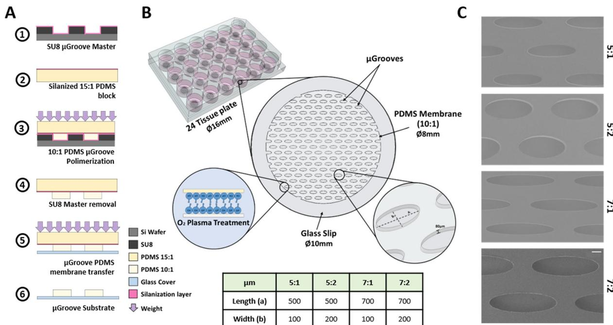
**Fig. 1**  $\mu$ Grooved substrates fabrication. (A). Schematic sequence of  $\mu$ Grooves fabrication. (B). Cells are confined within these microwells.  $\mu$ Grooves masters fabrication was designed to obtain features of 80  $\mu\text{m}$ -height. This condition was confirmed by stylus profilometer. (C). SEM images from the  $\mu$ Grooves. Scale bar: 100  $\mu\text{m}$ .
