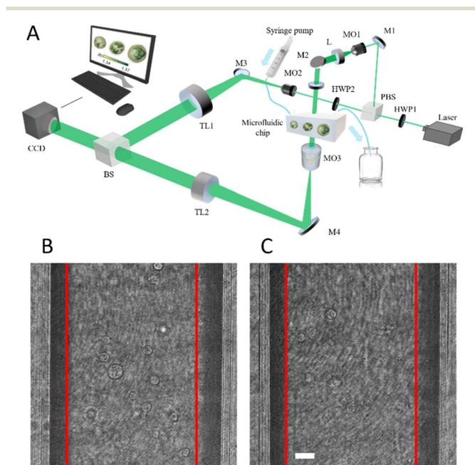
**Fig. 1** Opto-fluidic recording system. A) Sketch of the DH flow cytometer. L – lens; M – mirror; HWP – half-wave plate; PBS – polarizing beam splitter; MO – microscope objective; TL – tube lens; BS – beam splitter; CCD – camera. B and C) report 1024 × 1024 DH frames with flowing ISK and ISK-CisR cells, respectively, with highlighted in red the 1024 × 625 cut performed for feeding the Mask R-CNN. The scale bar is 20 μm.
