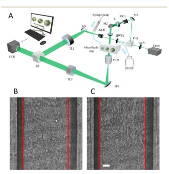
Fig. 1 Opto-fluidic recording system. A) Sketch of the DH flow cytometer. L – lens; M – mirror; HWP – half-wave plate; PBS – polarizing beam splitter; MO – microscope objective; TL – tube lens; BS – beam splitter; CCD – camera. B and C) report 1024  $\times$  1024 DH frames with flowing ISK and ISK-CisR cells, respectively, with highlighted in red the 1024  $\times$  625 cut performed for feeding the Mask R-CNN. The scale bar is 20  $\mu m$ .
