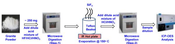
**Development of a simple and efficient two-step microwave-assisted digestion method for the determination of REEs, HFSEs and other elements in granite samples by ICP-OES**
