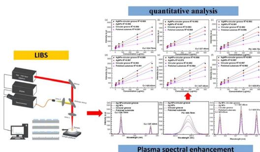
**High-sensitivity determination of heavy metal elements in water with circular grooves and nanoparticle-enhanced LIBS**
